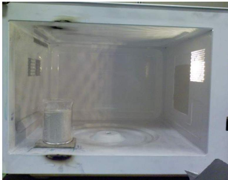
**Figure 2- 12: Picture indicating the position of the beaker within the DMO.**
