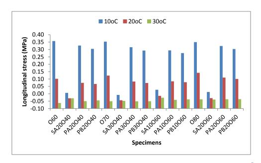
Figure 6.34: Longitudinal stress 4 mm above the crack top at 10oC, 20oC and  $30^{\circ}$ C with the load placed at the edge (Full bond)
