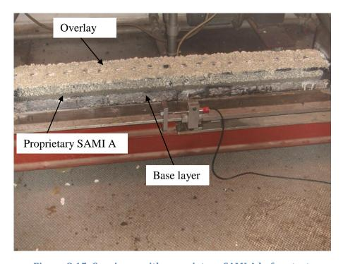
Figure 8.15: Specimen with proprietary SAMI A before test
