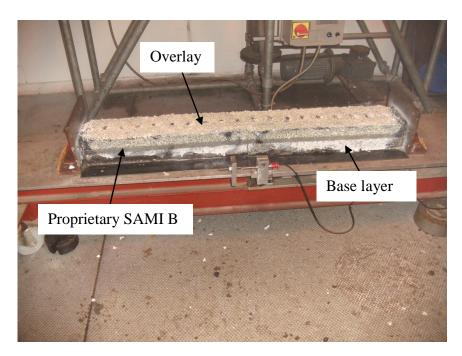
Figure 8.22: Specimen with proprietary SAMI B before test
