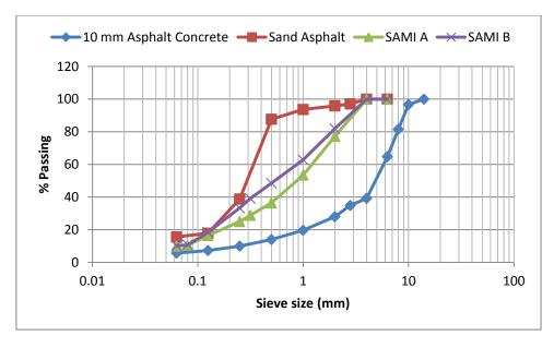
Figure 3.5: Particle size distribution for the blend of aggregates for overlay and SAMIs
