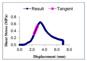
Figure A.4: Stress versus displacement graph for overlay-proprietary SAMI D interface at  $10^{\circ}$ C
