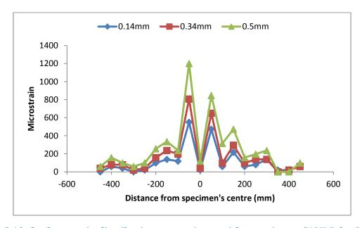
Figure 8.19: Surface strain distribution on specimen with proprietary SAMI B for 0.14mm, 0.34mm and maximum of 0.5mm crack openings
