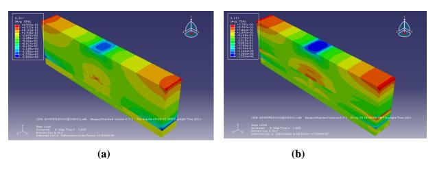
Figure 6.25: 20 mm proprietary SAMI B with 60 mm Overlay at 20°C with centre load (PB20060) (a) Full bond (b) Debond
