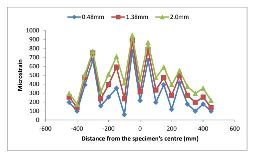
Figure 8.36: Surface strain distribution on specimen with proprietary SAMI D for 0.48mm, 1.38mm and maximum of 2mm crack openings
