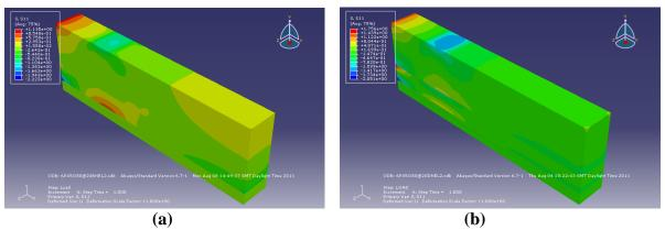
Figure 6.30: 80 mm Overlay at 20°C with edge load (080) (a) Full bond (b) Debond
