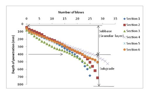
Figure 7.3: DCP test results
