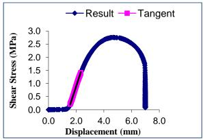
Figure A.8: Stress versus displacement graph for overlay-proprietary SAMI B interface at  $20^{\circ}\text{C}$
