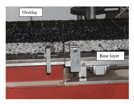
Figure 8.9: Control specimen before test
