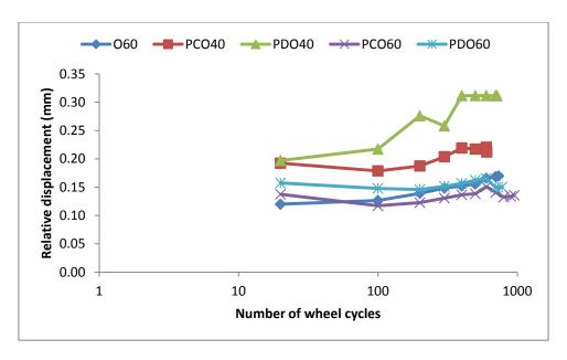
Figure 5.31: Displacement versus number of wheel cycles at 30°C with 1.35kN (0.6MPa) load applied for specimens with proprietary SAMIs C and D
