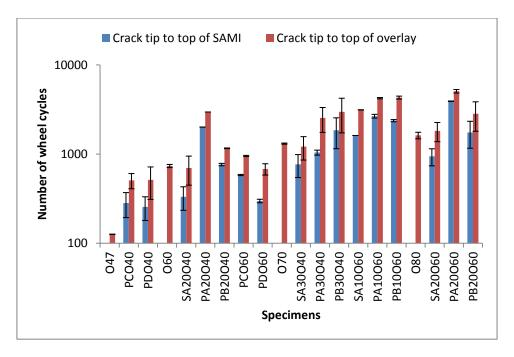
Figure 5.11: Number of wheel cycles to the top of SAMI and overlay at 30°C with 1.35kN load applied
