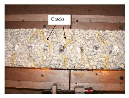
Figure 8.16: Specimen with proprietary SAMI A after test (centre)
