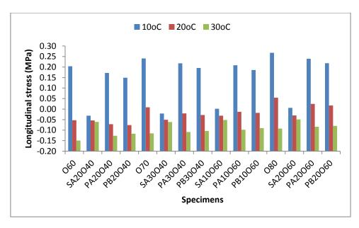
Figure 6.35: Longitudinal stress 4 mm above the crack top at 10°C, 20°C and 30°C with the load placed at the edge (Debond)
