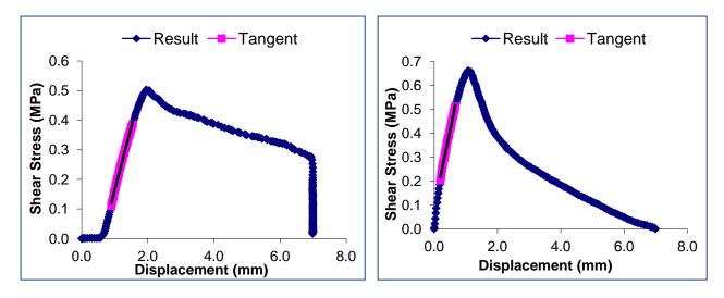
Figure B-9: Shear stress versus displacement for section 3 with 5 mm proprietary SAMI A before trafficking at 20°C
