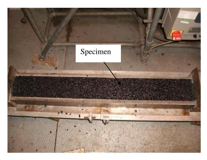
Figure 8.4: Thermal cracking testing device with the specimen in place
