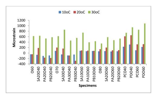
Figure 5.51: Strain at 20 mm from bottom of overlay and equivalent depth in control specimens under 2.4kN (1.1MPa) load at 10°C, 20°C and 30°C
