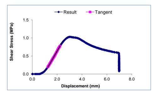
Figure B-8: Shear stress versus displacement for section 1 with 10 mm proprietary SAMI A after trafficking at  $20^{\circ}\mathrm{C}$
