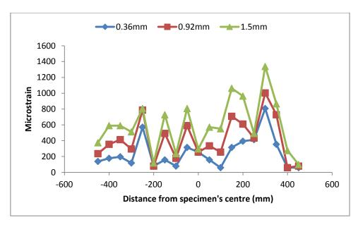
Figure 8.26: Surface strain distribution on specimen with proprietary SAMI C for 0.36mm, 0.92mm and maximum of 1.5mm crack openings
