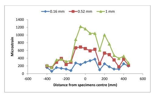
Figure 8.12: Surface strain distribution on specimen with proprietary SAMI A for 0.16mm, 0.52mm and maximum of 1.0mm crack openings
