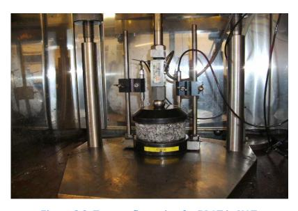
Figure 3.9: Test configuration for RLAT in NAT
