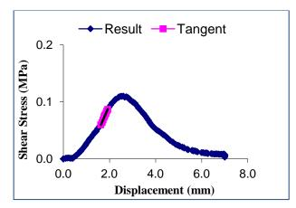
Figure A.15: Stress versus displacement graph for overlay-proprietary SAMI C interface at 30°C
