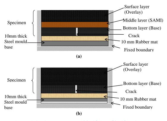
Figure 6.1: Specimen arrangement (a) with SAMI (b) without SAMI
