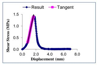
Figure A.12: Stress versus displacement graph for control (10 AC 40/60 -10AC 10/20) interface at  $20^{\circ}$ C
