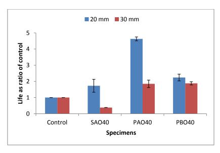
Figure 5.12: Number of wheel cycles to failure as ratio of control with 20 mm and 30 mm SAMIs and 40 mm overlay at 20°C and 2.4kN (1.1MPa)
