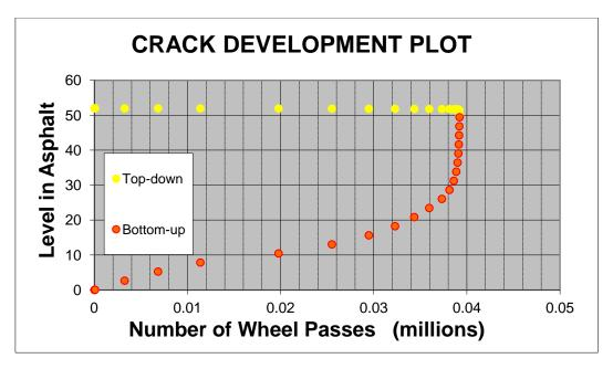
Figure 9.4: Graph of crack development for pavement with proprietary SAMI D
