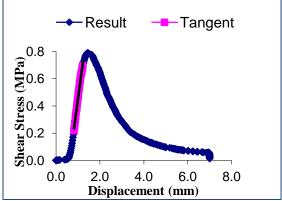
Figure A.3: Stress versus displacement graph for overlay-proprietary SAMI C interface at  $10^{\circ}$ C
