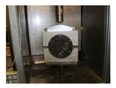
Figure 4.4: Leutner shear test equipment
