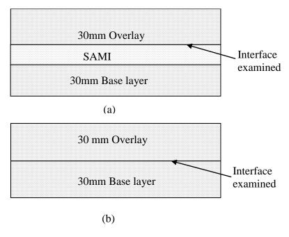
Figure 4.2: Cross-section of the system examined using Pull-off test (a) with SAMI (b) without SAMI
