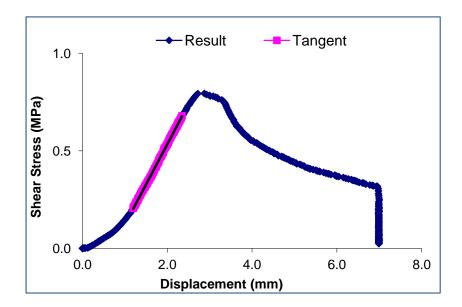
Figure B-10: Shear stress against displacement for section 3 with 5 mm proprietary SAMI A after trafficking at  $20^{\circ}$ C
