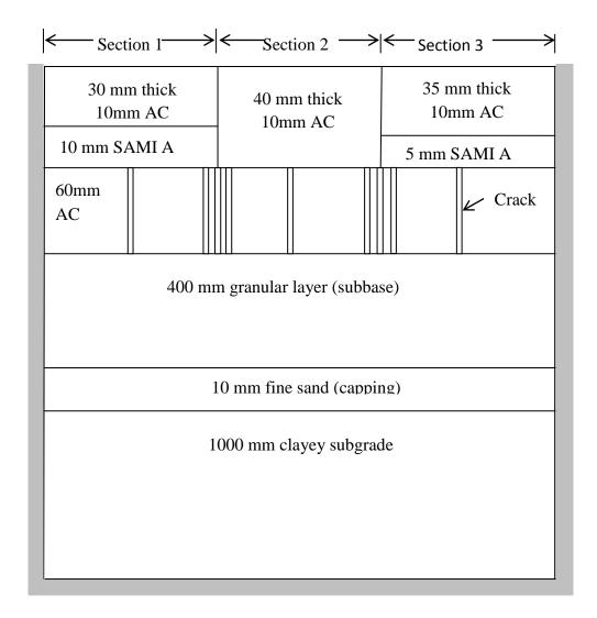
Figure 7.17: Pavement structure for sections 1, 2 and 3
