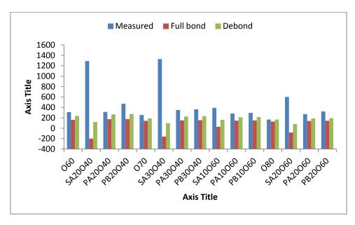
Figure 6.15: Strain at 4 mm above the crack top at 20°C
