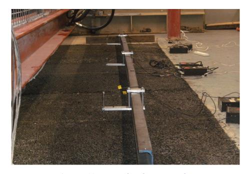
Figure 7.19: LVDTs placed across cracks
