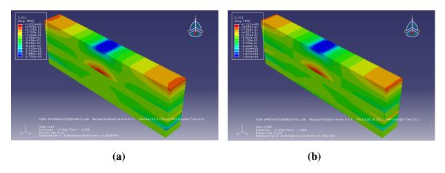
Figure 6.23: 20 mm sand asphalt with 60 mm Overlay at 20°C with centre load (SA20060) (a) Full bond (b) Debond
