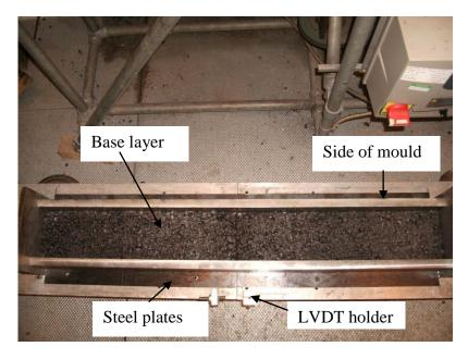
Figure 8.3: Thermal cycling testing device with the specimen's base layer, the end plates and the two side plates.
