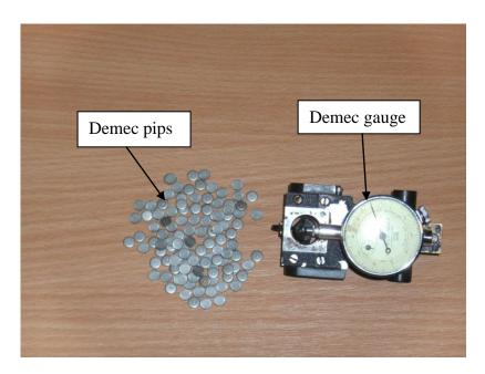
Figure 8.6: Demec gauge and pips
