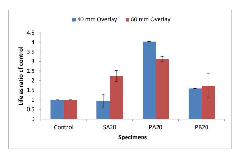
Figure 5.23: The number of wheel cycles to failure as ratio of control for specimens with 20mm SAMI and 40 mm and 60 mm overlay and 1.35kN load applied at 30°C
