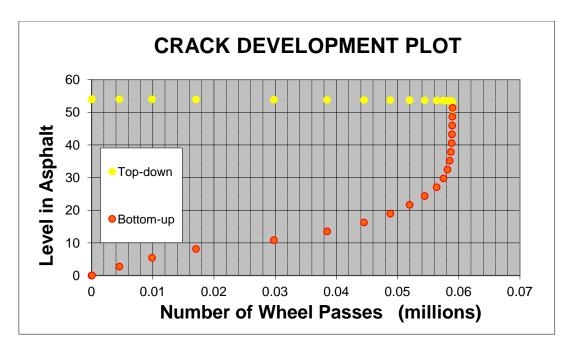
Figure 9.3: Graph of crack development for pavement with proprietary SAMI C
