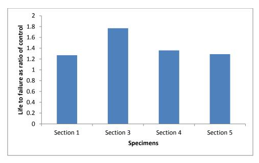
Figure 7.27: Life to failure as ratio of control for closely-spaced cracks
