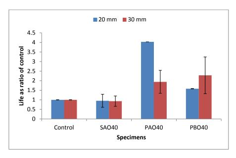
Figure 5.16: Number of wheel cycles to failure as ratio of control with 20 mm and 30 mm SAMIs and 40 mm overlay at 30°C and 1.35kN (0.6MPa)
