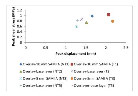
Figure 7.33: Peak shear stress versus peak displacement (mm)
