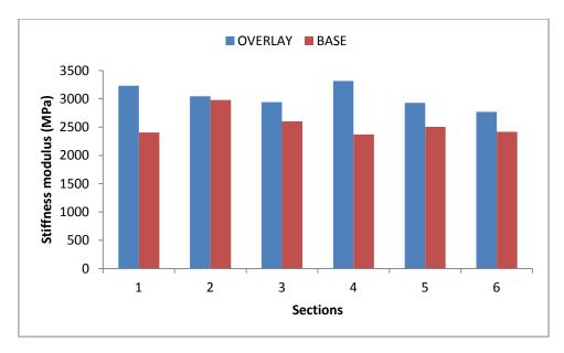
Figure 7.35: Stiffness modulus at 20°C
