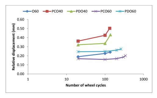
Figure 5.30: Displacement versus number of wheel cycles at 30°C with 2.4kN (1.1MPa) load applied for specimens with proprietary SAMIs C and D
