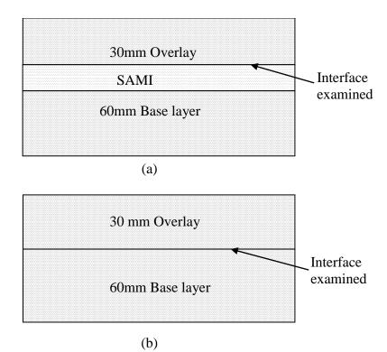
Figure 4.1: Cross-section of the system examined using Leutner shear test (a) with SAMI (b) without SAMI
