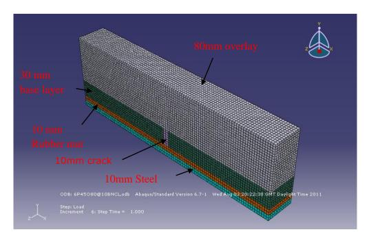
Figure 6.8: A typical model (Control) 80 mm overlay
