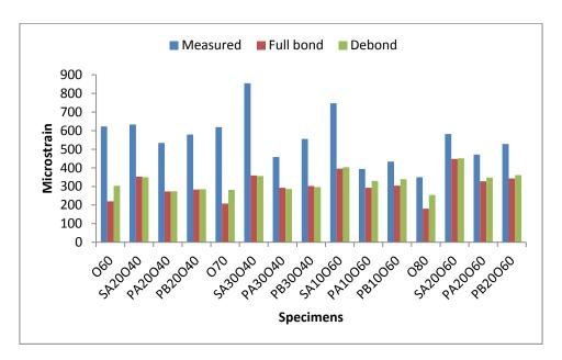
Figure 6.21: Strain at 20 mm from the bottom of the overlay at 30°C
