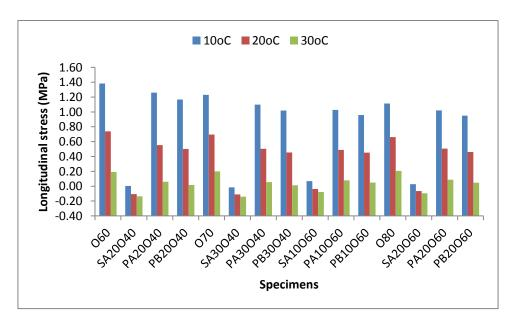
Figure 6.26: Longitudinal stress at crack tip at 10°C, 20°C and 30°C with the load placed at the centre (Full bond)
