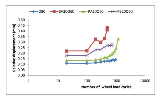
Figure 5.46: Displacement versus number of wheel cycles at 30°C with 2.4kN (1.1MPa) load applied for specimens with 20 mm SAMI and 60 mm overlay
