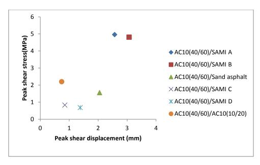
Figure 4.7: Peak shear stress versus peak shear displacement at 10°C
