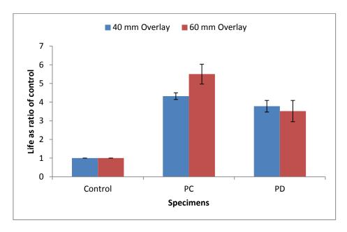
Figure 5.25: The number of wheel cycles to failure as ratio of control for specimens with SAMIs C and D and 40 mm and 60 mm overlay and 2.4kN load applied at 20°C
