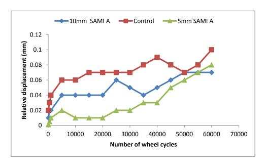
Figure 7.29: Relative displacement for wheel path 1
