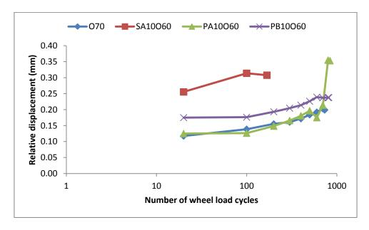
Figure 5.42: Displacement versus number of wheel cycles at 30°C with 2.4kN (1.1MPa) load applied for specimens with 10 mm SAMI and 60 mm overlay
