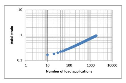
Figure 7.5: Repeated load axial test results
