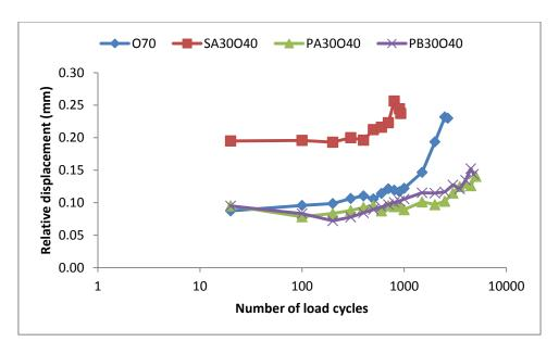
Figure 5.37: Displacement versus number of wheel cycles at 20°C with 2.4kN (1.1MPa) load applied for specimens with 30 mm SAMI and 40 mm overlay
