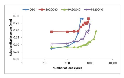
Figure 5.33: Displacement versus number of wheel cycles at 20°C with 2.4kN (1.1MPa) load applied for specimens with 20 mm SAMI and 40 mm overlay
