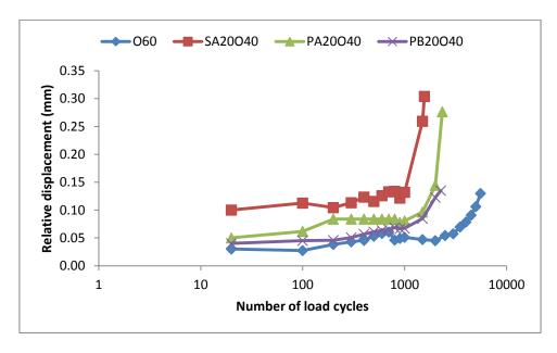
Figure 5.32: Displacement versus number of wheel cycles at 10°C with 2.4kN (1.1MPa) load applied for specimens with 20 mm SAMI and 40 mm overlay
