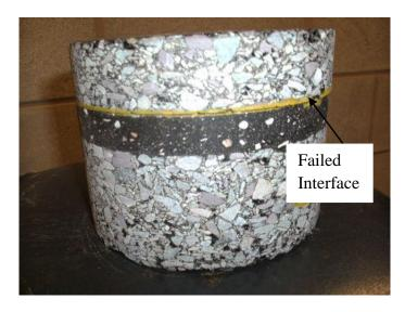
Figure 4.11: A typical failed interface after test
