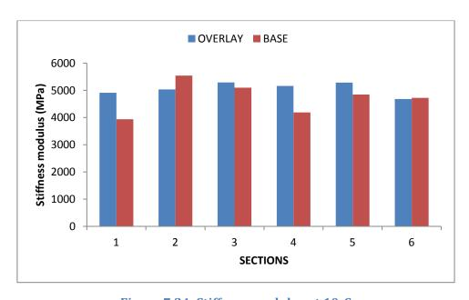
Figure 7.34: Stiffness modulus at 10°C
