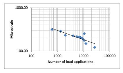
Figure 7.4: Fatigue line of the asphalt
