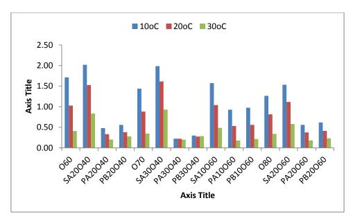
Figure 6.29: Longitudinal stress at bottom of overlay at 10°C, 20°C and 30°C with the load placed at the centre (Debond)
