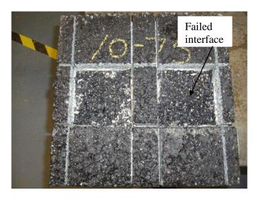
Figure 4.15: A typical failed interface after test
