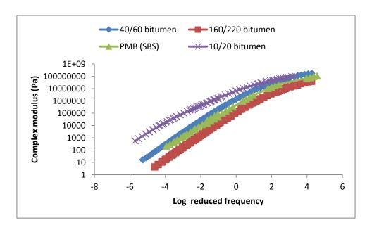
Figure 3.2: Complex modulus master curves at reference temperature of 25°C
