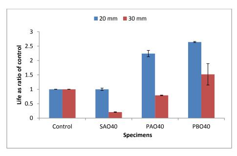
Figure 5.14: Number of wheel cycles to failure as ratio of control with 20 mm and 30 mm SAMIs and 40 mm overlay at 30°C and 2.4kN (1.1MPa)
