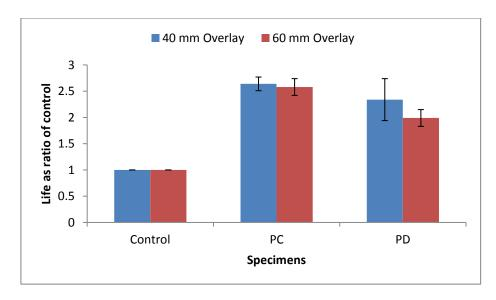
Figure 5.26: The number of wheel cycles to failure as ratio of control for specimens with SAMIs C and D and 40 mm and 60 mm overlay and 2.4kNload applied at 30°C
