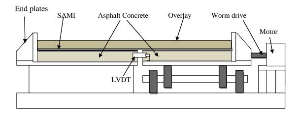
Figure 8.1: Schematic of the thermal cycling device (Baxter, 2001)
