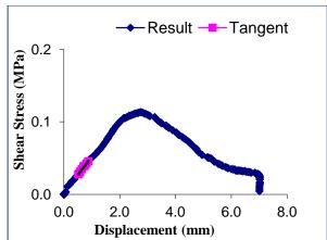
Figure A.16: Stress versus displacement graph for overlay-proprietary SAMI D interface at  $30^{\circ}\text{C}$
