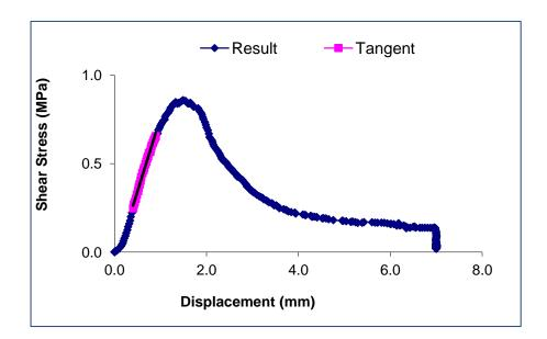
Figure B-12: Shear stress against displacement for section 2 with no SAMI (Control) after trafficking at  $20^{\circ}\text{C}$
