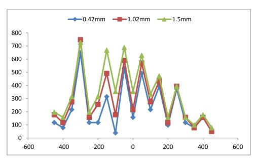
Figure 8.35: Surface strain distribution on specimen with proprietary SAMI D for 0.42mm, 1.02mm and maximum of 1.5mm crack openings
