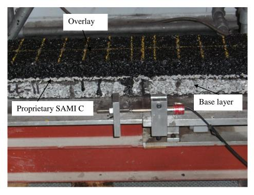
Figure 8.30: Specimen with proprietary SAMI C before test
