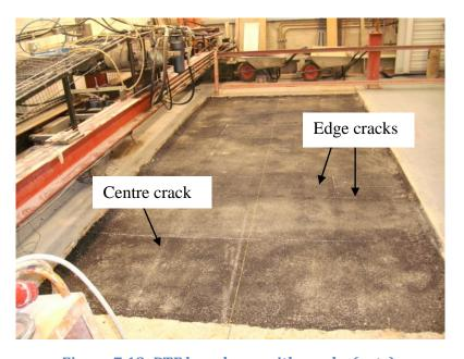
Figure 7.13: PTF base layer with cracks (cuts)
