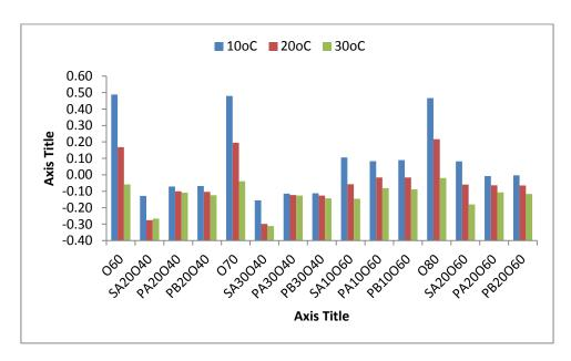
Figure 6.36: Longitudinal stress at bottom of overlay at 10°C, 20°C and 30°C with the load placed at the edge (Full bond)
