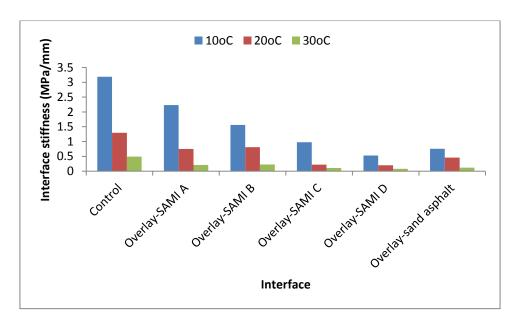
Figure 4.10: Shear stiffness of the interface
