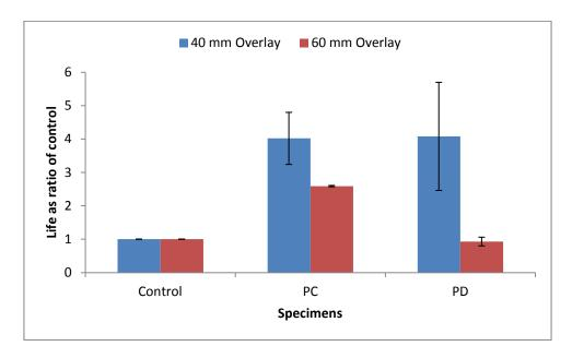
Figure 5.27: The number of wheel cycles to failure as ratio of control for specimens with SAMIs C and D and 40 mm and 60 mm overlay and 1.35kN load applied at 30°C
