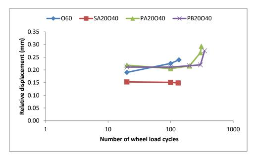
Figure 5.34: Displacement versus number of wheel cycles at 30°C with 2.4kN (1.1MPa) load applied for specimens with 20 mm SAMI and 40 mm overlay
