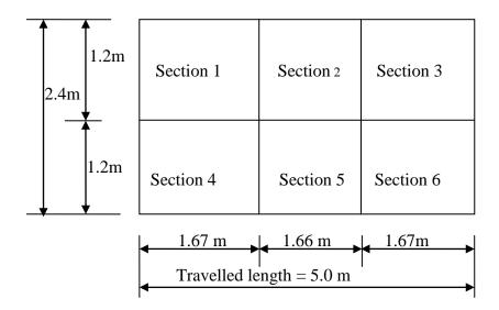
Figure 7.11: Schematic of the PTF pavement sections
