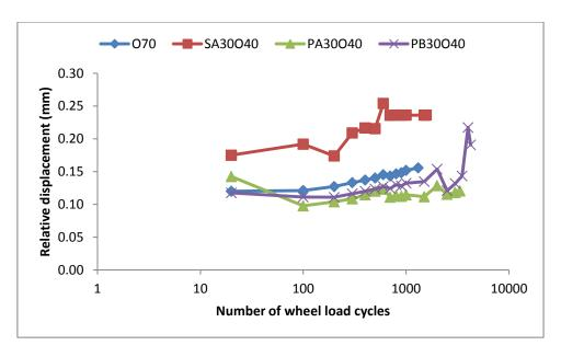
Figure 5.39: Displacement versus number of wheel cycles at 30°C with 1.35MPa (0.6MPa) load applied for specimens with 30 mm SAMI and 40 mm overlay
