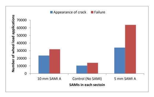
Figure 7.22: Number of load applications to the appearance of cracks and failure for wheel path 1
