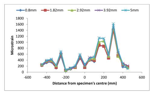
Figure 8.29: Surface strain distribution on specimen with proprietary SAMI C for 0.8mm, 1.82mm, 2.92mm, 3.92mm and maximum of 5.0mm crack openings
