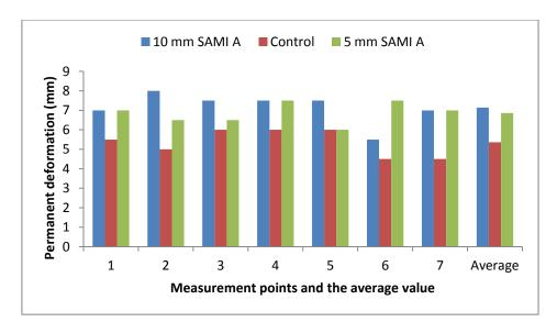
Figure 7.31: Permanent deformation for wheel path 1
