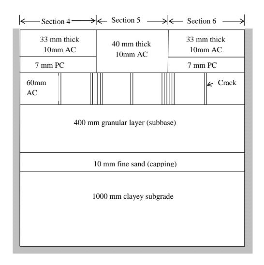
Figure 7.18: Pavement structure for sections 4, 5 and 6
