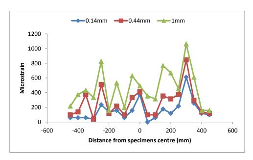
Figure 8.25: Surface strain distribution on specimen with proprietary SAMI C for 0.14mm, 0.44mm and maximum of 1.0mm crack openings
