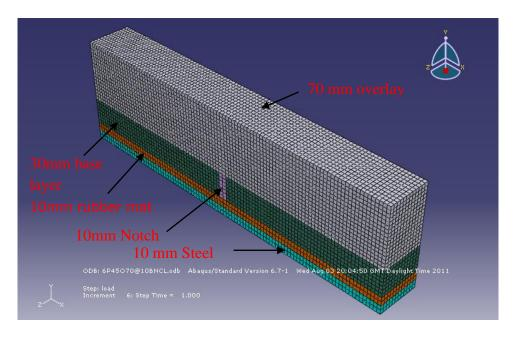
Figure 6.7: A typical model (Control) 70 mm overlay
