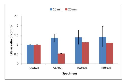
Figure 5.13: Number of wheel cycles to failure as ratio of control with 10 mm and 20 mm SAMIs and 60 mm overlay at 20°C and 2.4kN (1.1MPa)
