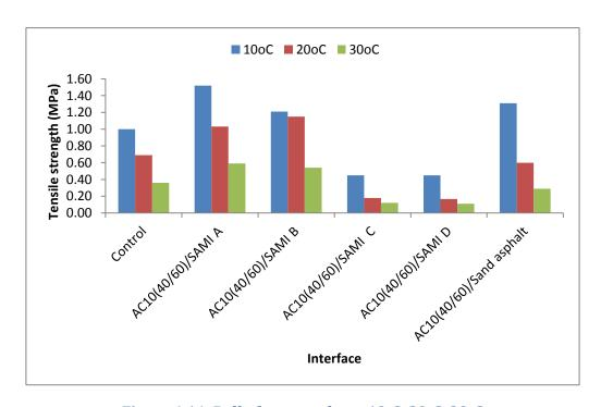
Figure 4.14: Pull of test results at 10°C, 20°C, 30°C
