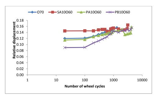
Figure 5.43: Displacement versus number of wheel cycles at 30°C with 1.35kN (0.6MPa) load applied for specimens with 10 mm SAMI and 60 mm overlay
