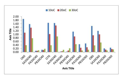
Figure 6.28: Longitudinal stress at bottom of overlay at 10°C, 20°C and 30°C with the load placed at the centre (Full bond)
