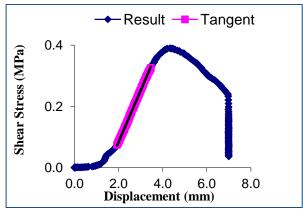
Figure A.17: Stress versus displacement graph for overlay-proprietary sand asphalt interface at  $30^{\circ}\mathrm{C}$
