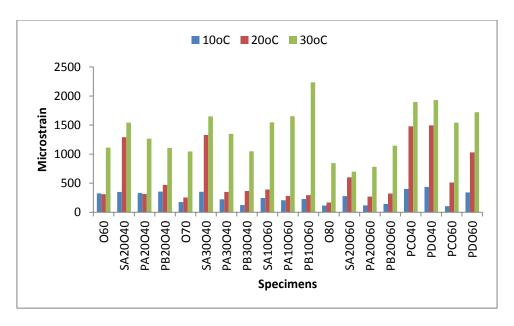
Figure 5.50: Strain at 4 mm above the crack top under 2.4kN (1.1MPa) load at 10°C, 20°C and 30°C
