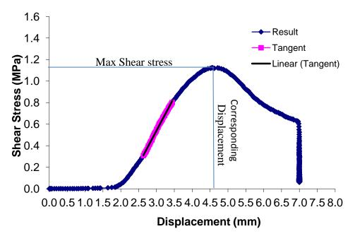
Figure 4.6: A typical shear stress versus displacement graph
