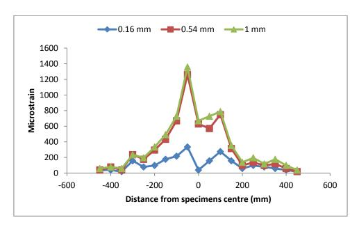
Figure 8.43: Surface strain distribution on specimen with sand asphalt for 0.16mm, 0.54mm and maximum of 1mm crack openings
