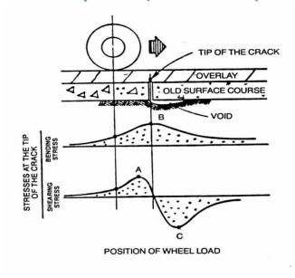
Figure 1.4: Stresses induced at crack tip by wheel load (Lytton, 1989)
