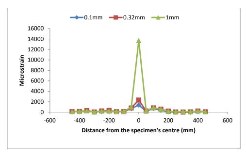
Figure 8.8: Surface strain distribution on control specimen for 0.1mm, 0.32mm and maximum of 1.0mm crack openings
