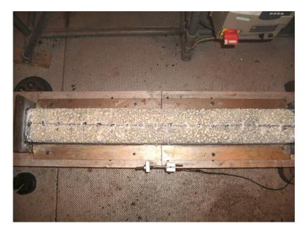
Figure 8.46: Specimen with sand asphalt at the start of test
