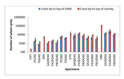
Figure 5.8: Number of wheel cycles to the top of SAMI and overlay at 10°C with 2.4kN load applied
