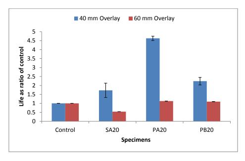
Figure 5.21: The number of wheel cycles to failure as ratio of control for specimens with 20mm SAMI and 40 mm and 60 mm overlay and 2.4kN load applied at 20°C
