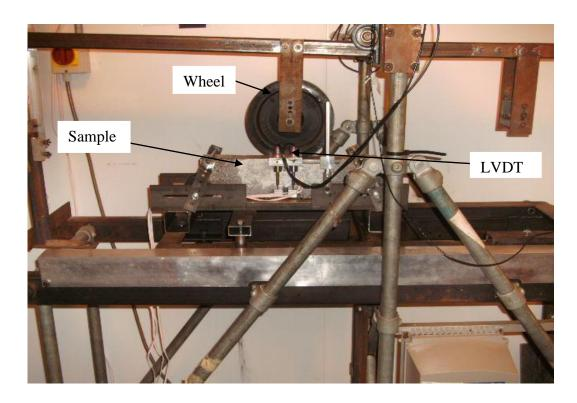
Figure 5.5: Wheel tracking machine with sample
