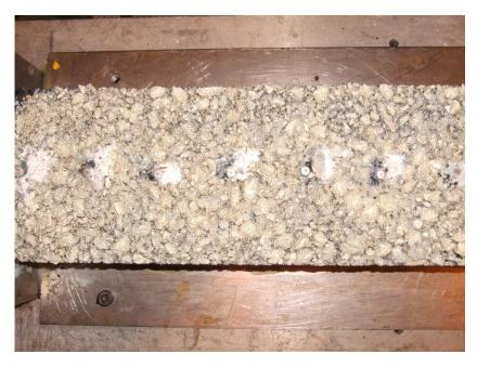
Figure 8.18: Specimen with proprietary SAMI A after test (left)
