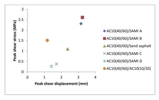
Figure 4.8: Peak shear stress versus peak shear displacement at 20°C
