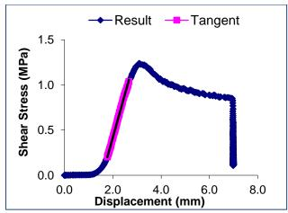
Figure B-7: Shear stress versus displacement for section 1 with 10 mm proprietary SAMI A before trafficking at  $20^{\circ}$ C
