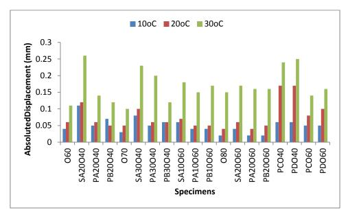
Figure 5.48: Initial absolute displacement of the specimens under 2.4kN load at  $10^{\circ}$ C,  $20^{\circ}$ C and  $30^{\circ}$ C
