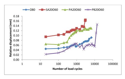
Figure 5.45: Displacement versus number of wheel cycles at 20°C with 2.4kN (1.1MPa) load applied for specimens with 20 mm SAMI and 60 mm overlay
