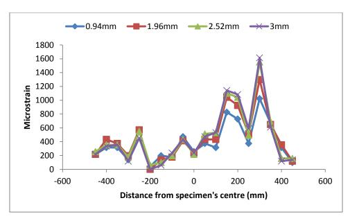
Figure 8.28: Surface strain distribution on specimen with proprietary SAMI C for 0.94mm, 1.96mm, 2.52mm and maximum of 3.0mm crack openings
