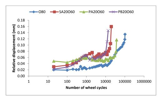
Figure 5.44: Displacement versus number of wheel cycles at 10°C with 2.4kN (1.1MPa) load applied for specimens with 20 mm SAMI and 60 mm overlay
