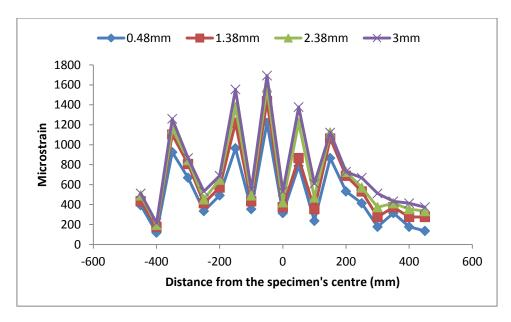
Figure 8.37: Surface strain distribution on specimen with proprietary SAMI D for 0.48mm, 1.38mm, 2.38mm, and maximum of 3mm crack openings
