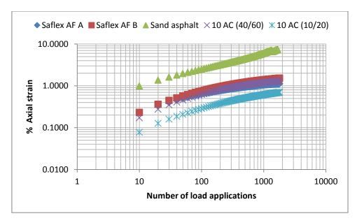
Figure 3.10: Permanent deformation results
