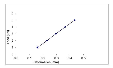
Figure 3.4: Load-displacement curve for the rubber mat
