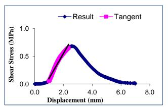
Figure A.18: Stress versus displacement graph for control (10 AC 40/60 -10AC 10/20) interface at  $30^{\rm o}{\rm C}$
