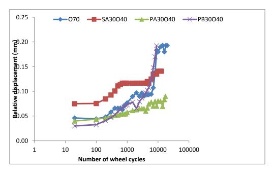
Figure 5.36: Displacement versus number of wheel cycles at 10°C with 2.4kN (1.1MPa) load applied for specimens with 30 mm SAMI and 40 mm overlay
