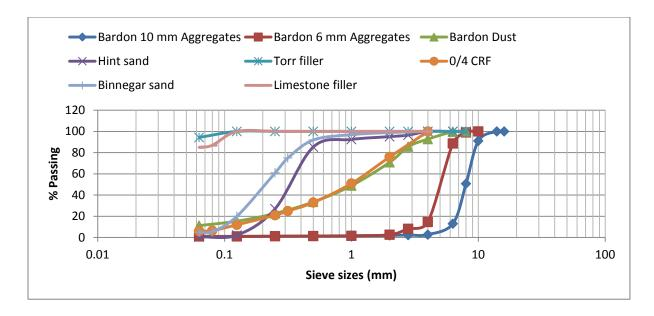
Figure 3.1: Particle size distribution of the aggregates
