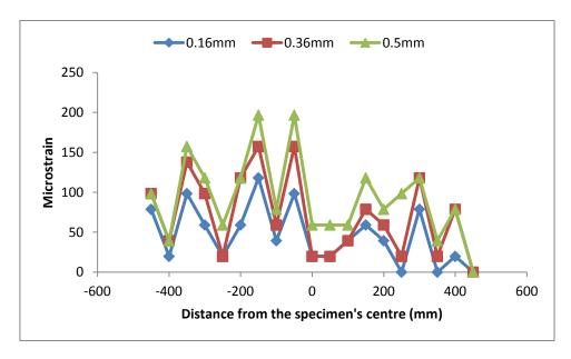
Figure 8.33: Surface strain distribution on specimen with proprietary SAMI D for 0.16mm, 0.36mm and maximum of 0.5mm crack openings
