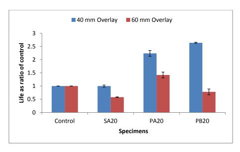
Figure 5.22: The number of wheel cycles to failure as ratio of control for specimens with 20mm SAMI and 40 mm and 60 mm overlay and 2.4kN load applied at 30°C
