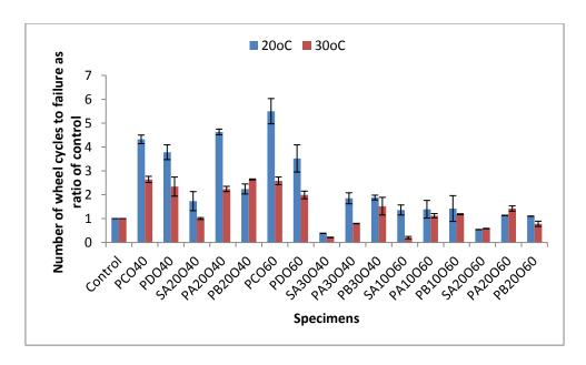
Figure 5.20: The number of wheel cycles to failure as ratio of control with 2.4kN load applied at 20°C and 30°C
