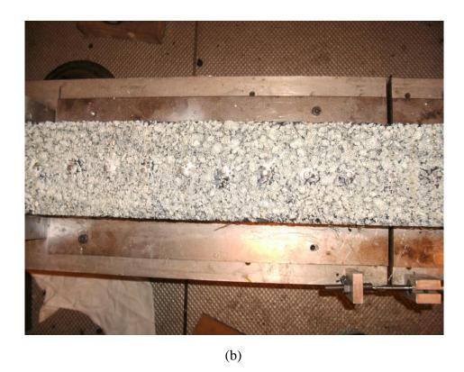
Figure 8.32: Specimen with proprietary SAMI C after test (left)
