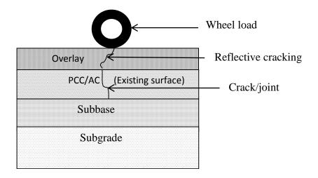
Figure 1.2: Schematic of reflective cracking in pavement
