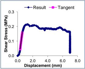
Figure B-11: Shear stress against displacement for section 2 with no SAMI (Control) before trafficking at  $20^{\circ}\text{C}$
