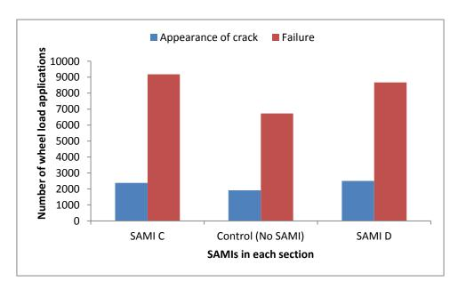
Figure 7.26: Number of load applications to the appearance of cracks and failure for wheel path 2 for closely spaced cracks
