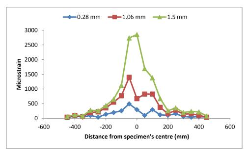
Figure 8.44: Surface strain distribution on specimen with sand asphalt for 0.28mm, 1.06mm and maximum of 1.5mm crack openings
