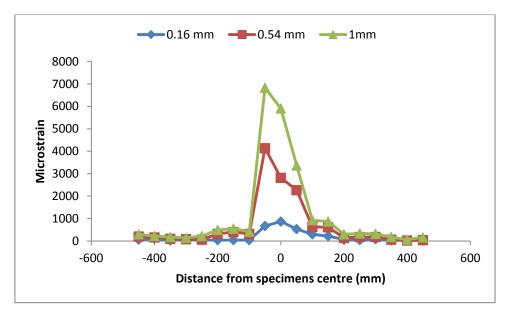
Figure 8.20: Surface strain distribution on specimen with proprietary SAMI B for 0.16mm, 0.54mm and maximum of 1.0mm crack openings
