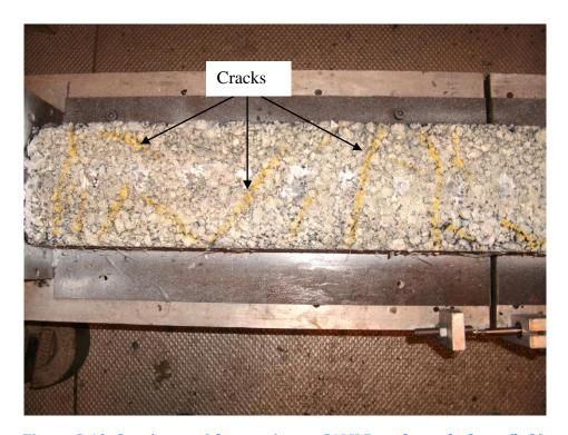
Figure 8.40: Specimen with proprietary SAMI D at the end of test (left)
