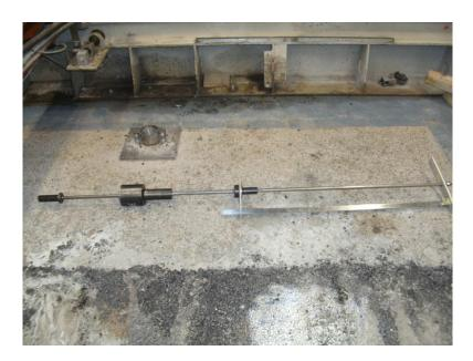
Figure 7.2: Dynamic cone penetrometer
