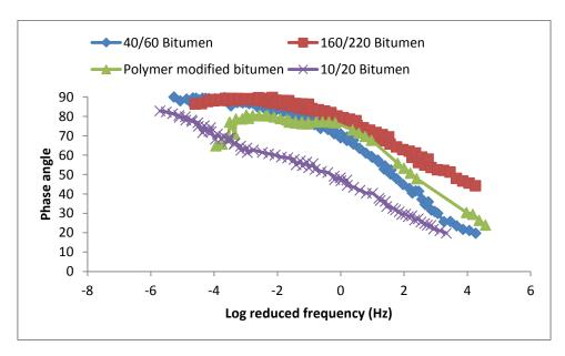
Figure 3.3: Phase angle master curves at reference temperature of 25°C
