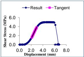
Figure A.1: Stress versus displacement graph for overlay-proprietary SAMI A interface at  $10^{\circ} \text{C}$
