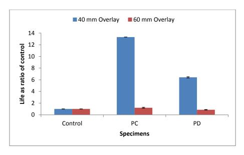
Figure 5.24: The number of wheel cycles to failure as ratio of control for specimens with SAMIs C and D and 40 mm and 60 mm overlay and 2.4kN load applied at 10°C
