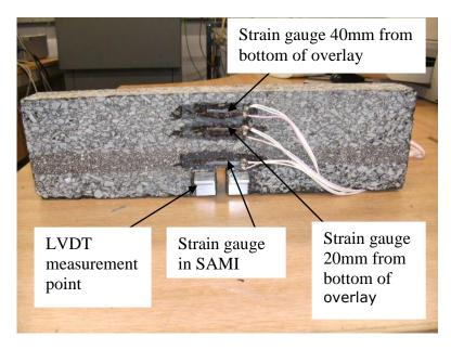
Figure 5.4: A typical beam with strain gauges and LVDT measurement points
