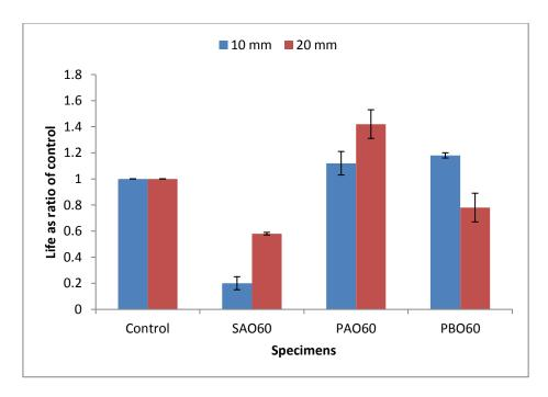
Figure 5.15: Number of wheel cycles to failure as ratio of control with 10 mm and 20 mm SAMIs and 60 mm overlay at  $30^{\circ}$ C and 2.4kN (1.1MPa)
