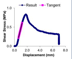
Figure B-13: Shear stress versus displacement for section 5 with no SAMI (Control) before trafficking at  $20^{\circ}\text{C}$
