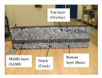
Figure 5.3: A typical beam with notch for wheel tracking test
