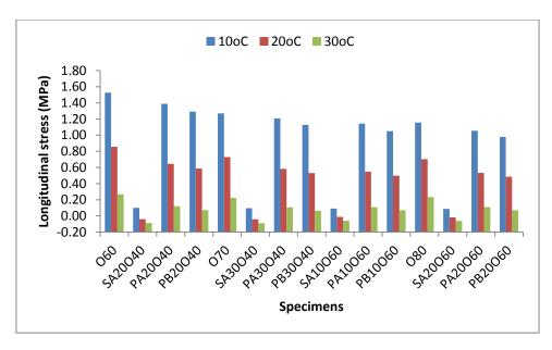
Figure 6.27: Longitudinal stress at crack tip at 10°C, 20°C and 30°C with the load placed at the centre (Debond)
