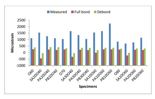
Figure 6.16: Strain at 4 mm above the crack top at 30°C
