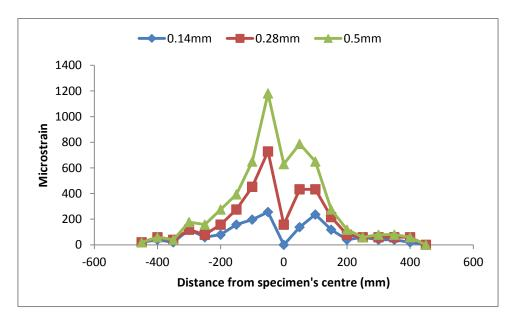
Figure 8.42: Surface strain distribution on specimen with sand asphalt for 0.14mm, 0.28mm and maximum of 0.5mm crack openings
