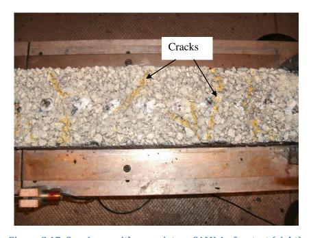
Figure 8.17: Specimen with proprietary SAMI A after test (right)
