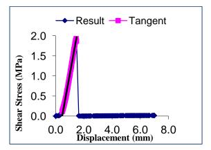
Figure A.6: Stress versus displacement graph for control (10 AC 40/60-10AC 10/20) interface at  $10^{\circ}$ C
