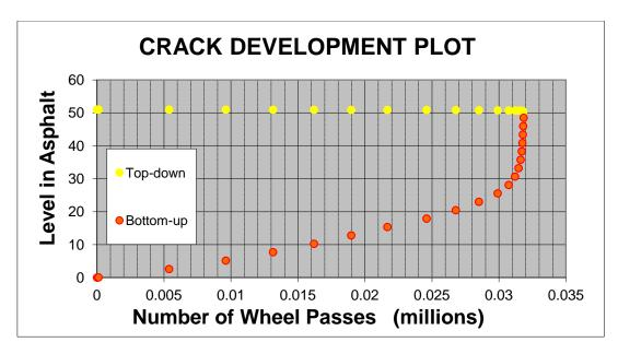
Figure 9.2: Graph of crack development for cracked pavement with 15 mm proprietary SAMI A  $\,$
