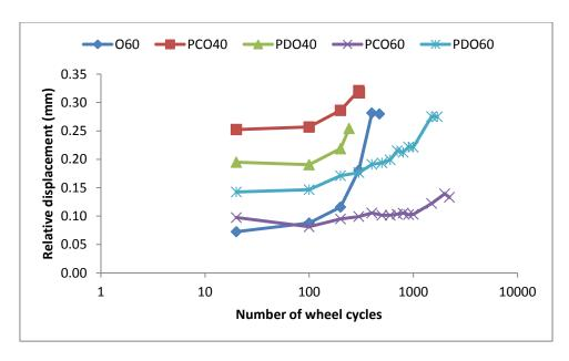
Figure 5.29: Displacement versus number of wheel cycles at 20°C with 2.4kN (1.1MPa) load applied for specimens with proprietary SAMIs C and D
