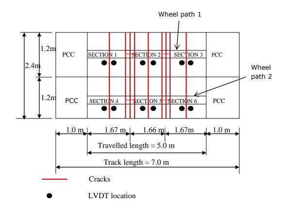
Figure 7.20: Wheel paths and LVDTs' locations
