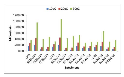
Figure 6.18: Strain at the bottom of the overlay (Debond)
