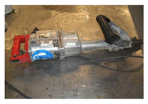
Figure 7.15: Vibrating hammer (Kango)
