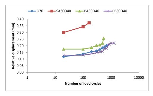
Figure 5.38: Displacement versus number of wheel cycles at 30°C with 2.4kN (1.1MPa) load applied for specimens with 30 mm SAMI and 40 mm overlay
