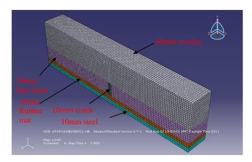
Figure 6.6: A typical model (Control) 60 mm overlay
