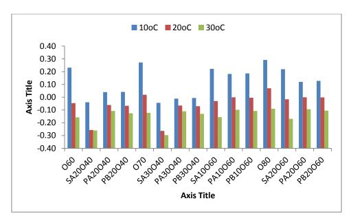
Figure 6.37: Longitudinal stress at bottom of overlay at 10°C, 20°C and 30°C with the load placed at the edge (Debond)
