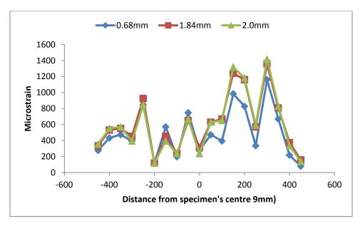
Figure 8.27: Surface strain distribution on specimen with proprietary SAMI C for 0.68mm, 1.84mm and maximum of 2.0mm crack openings
