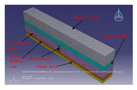
Figure 6.5: A typical model with 20 mm SAMI and 40 mm overlay
