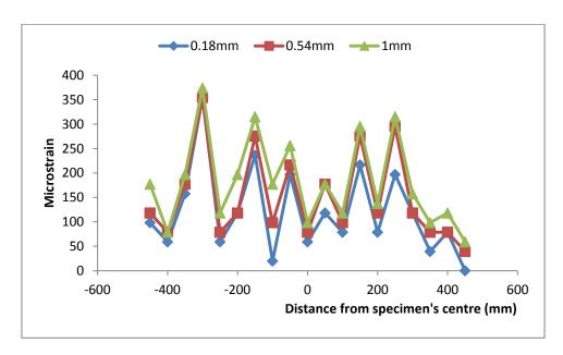
Figure 8.34: Surface strain distribution on specimen with proprietary SAMI D for 0.18mm, 0.54mm and maximum of 1mm crack openings
