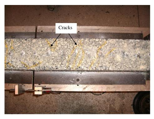
Figure 8.41: Specimen with proprietary SAMI D at the end of test (right)
