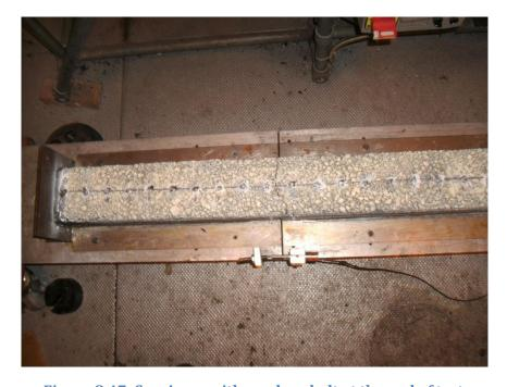
Figure 8.47: Specimen with sand asphalt at the end of test
