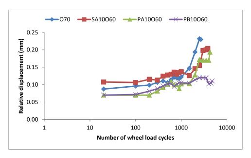
Figure 5.41: Displacement versus number of wheel cycles at 20°C with 2.4kN (1.1MPa) load applied for specimens with 10 mm SAMI and 60 mm overlay
