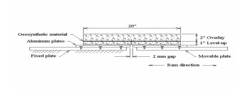
Figure 2.2: Schematic of TTI overlay tester (Cleveland et al, 2002)
