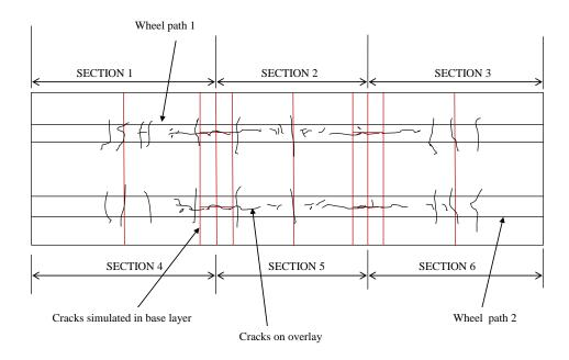
Figure 7.28: Crack patterns on wheel paths 1 and 2
