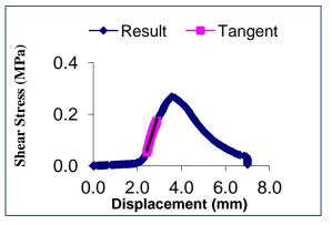
Figure A.9: Stress versus displacement graph for overlay- proprietary SAMI C interface at 20°C
