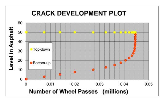
Figure 9.1: Graph of crack development for cracked pavement with 6 mm proprietary SAMI A  $\,$
