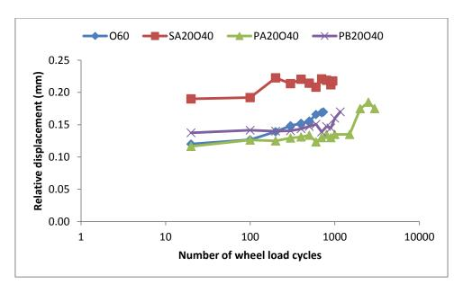
Figure 5.35: Displacement versus number of wheel cycles at 30°C with 1.35kN (0.6MPa) load applied for specimens with 20 mm SAMI and 40 mm overlay
