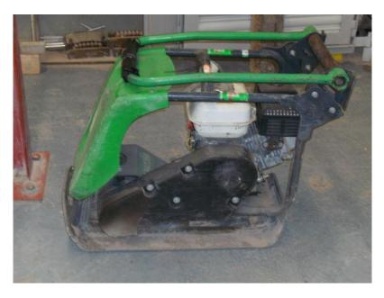
Figure 7.7: Vibrating plate
