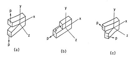
Figure 1.5: Modes of cracking (a) mode I (b) mode II and (c) mode III (Hughes, 1986)
