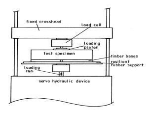
Figure 2.1: Beam testing arrangement (Caltabiano, 1990)
