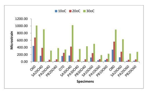
Figure 6.17: Strain at the bottom of the overlay (Full Bond)
