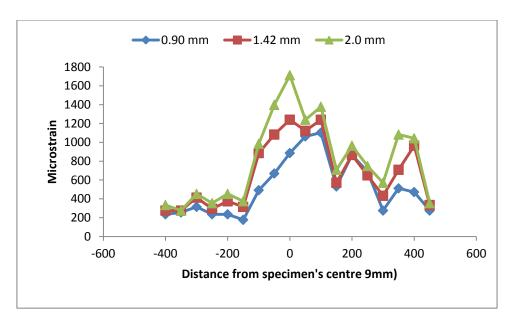
Figure 8.14: Surface strain distribution on specimen with proprietary SAMI A for 0.90mm, 1.42mm and maximum of 2.0mm crack openings
