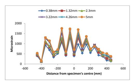
Figure 8.38: Surface strain distribution on specimen with proprietary SAMI D for 0.38mm, 1.32mm, 2.30mm, 3.22mm, 4.26mm and maximum of 5mm crack openings
