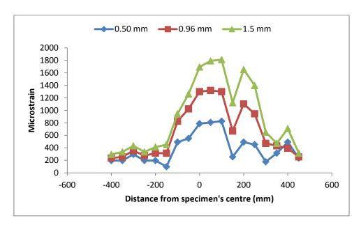
Figure 8.13: Surface strain distribution on specimen with proprietary SAMI A for 0.5mm, 0.96mm and maximum of 1.5mm crack openings
