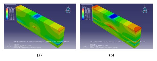
Figure 6.22: 80 mm Overlay at 20°C with centre load (080) (a) Full bond (b) Debond
