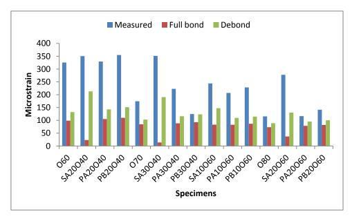
Figure 6.14: Strain at 4 mm above the crack top at 10°C
