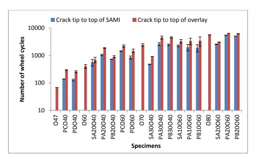
Figure 5.9: Number of wheel cycles to the top of SAMI and overlay at 20°C with 2.4kN load applied
