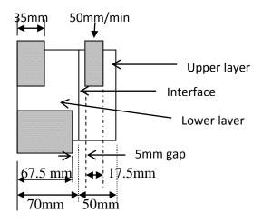
Figure 4.3: Schematic of the shear test equipment
