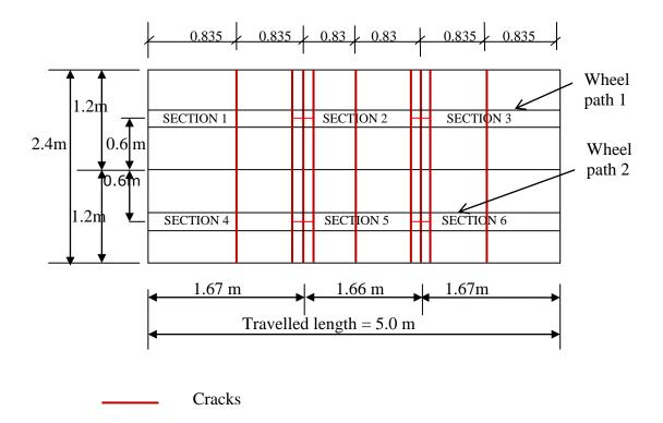
Figure 7.12: Simulated cracks in PTF sections
