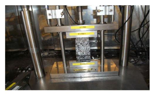
Figure 3.7: Test configuration for ITFT in NAT
