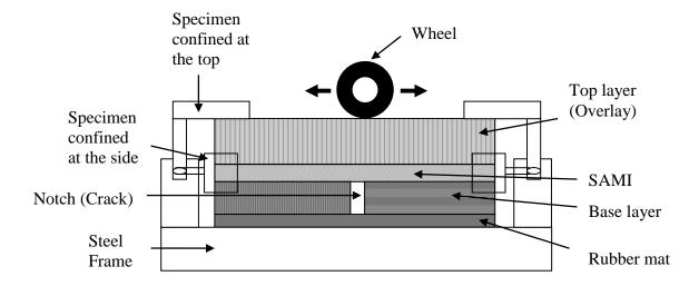
Figure 5.1: Schematic of the wheel tracking test
