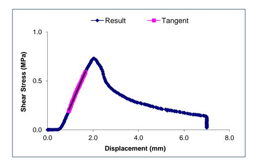
Figure B-14: Shear stress against displacement for section 5 with no SAMI (Control) after trafficking at  $20^{\circ}$ C
