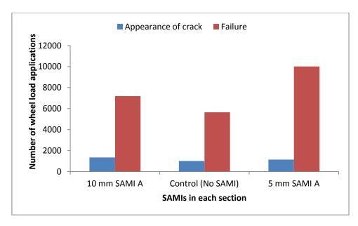
Figure 7.25: Number of load applications to the appearance of cracks and failure for wheel path 1 for closely spaced cracks
