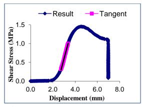
Figure A.5: Stress versus displacement graph for overlay-proprietary sand asphalt interface at 10°C
