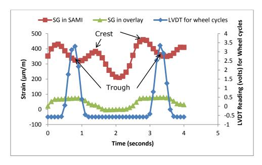
Figure 5.7: A typical strain readings analysis
