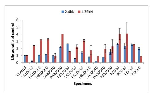
Figure 5.18: The number of wheel cycles to failure as ratio of control with 2.4kN and 1.35kN loads applied at 30°C
