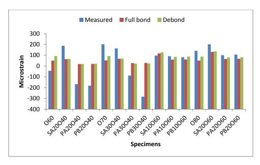
Figure 6.20: Strain at 20 mm from the bottom of the overlay at 20°C
