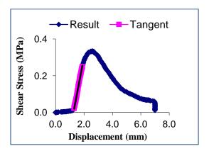
Figure A.10: Stress versus displacement graph for overlay-proprietary SAMI D interface at 20°C
