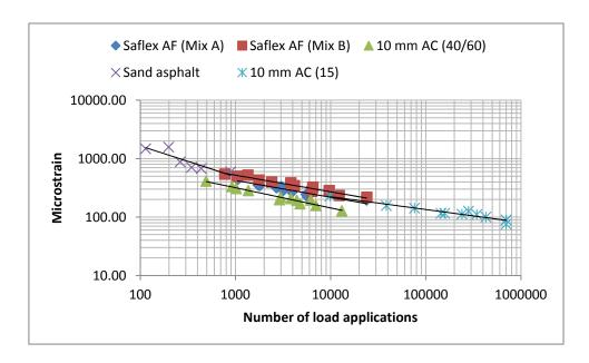
Figure 3.8: Fatigue lines for the bituminous mixtures
