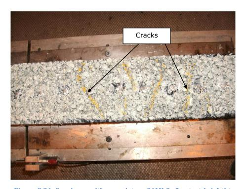
Figure 8.31: Specimen with proprietary SAMI C after test ( right) t
