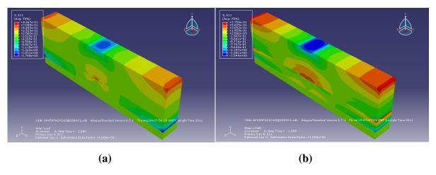
Figure 6.24: 20 mm proprietary SAMI A with 60 mm Overlay at 20°C with centre load (PA20060) (a) Full bond (b) Debond
