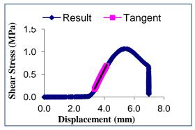
Figure A.11: Stress versus displacement graph for overlay-proprietary sand asphalt interface at 20°C
