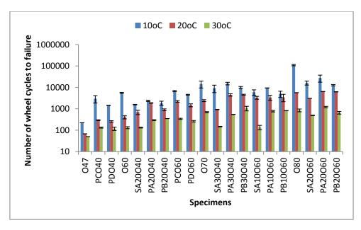
Figure 5.19: Number of wheel cycles to failure at 10°C, 20°C and 30°C under a load of 2.4kN (1.1MPa)
