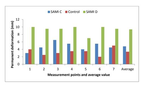
Figure 7.32: Permanent deformation for wheel path 2
