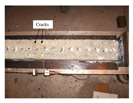
Figure 8.23: Specimen with proprietary SAMI B after test
