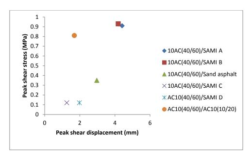
Figure 4.9: Peak shear stress versus peak shear displacement at 30°C
