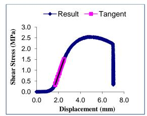
Figure A.7: Stress versus displacement graph for overlay-proprietary SAMI A interface at 20°C
