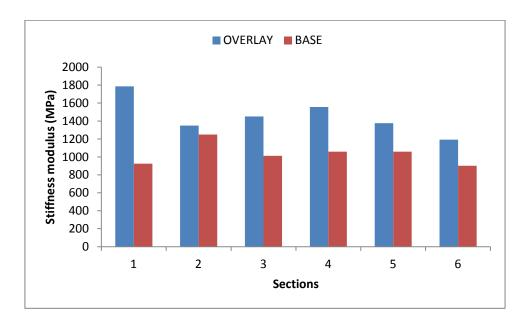
Figure 7.36: Stiffness modulus at 30°C
