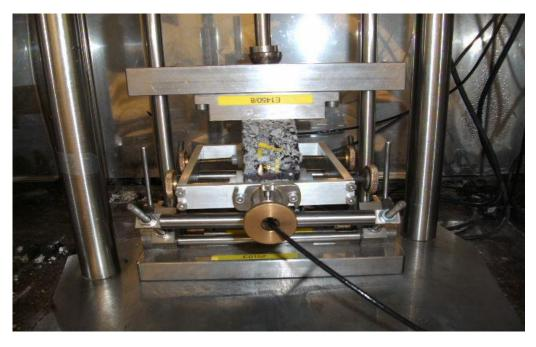
Figure 3.6: Test configuration for ITSM in NAT
