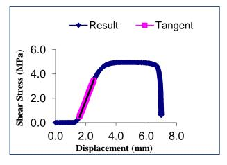
Figure A.2: Stress versus displacement graph for overlay-proprietary SAMI B interface at 10°C
