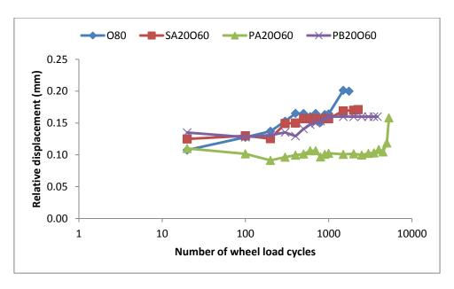
Figure 5.47: Displacement versus number of wheel cycles at 30°C with 1.35kN (0.6MPa) load applied for specimens with 20 mm SAMI and 60 mm overlay
