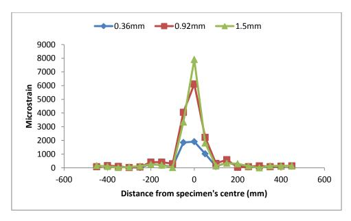
Figure 8.21: Surface strain distribution on specimen with proprietary SAMI B for 0.36mm, 0.92mm and maximum of 1.5mm crack openings
