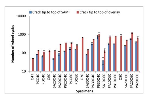
Figure 5.10: Number of wheel cycles to the top of SAMI and overlay at 30°C with 2.4kN load applied
