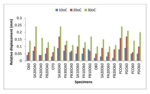
Figure 5.49: Initial relative displacement of the specimens under 2.4kN load at 10°C, 20°C and 30°C
