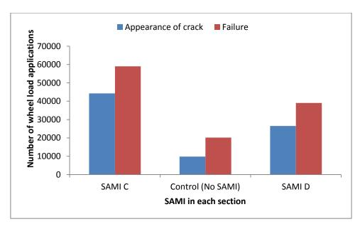
Figure 7.23: Number of load applications to the appearance of cracks and failure for wheel path 2
