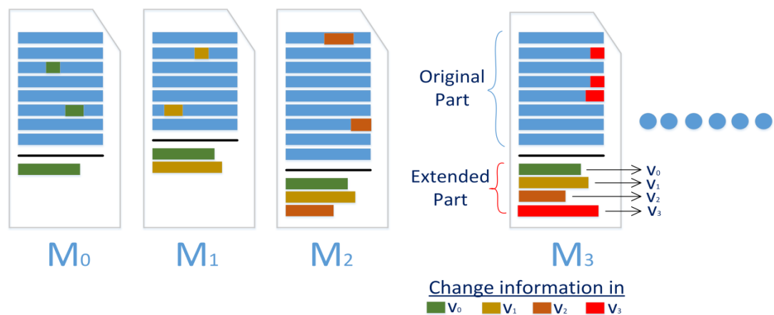
Figure 5.7: Graphical representation of original and extended parts in IFC.
