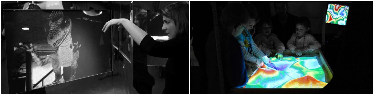
Fig. 4.3.1-3: a) SAR system for dinosaur exhibition, the visitors input is provided by haptics; b) The change in the deformable surface is the result of the user input (Mitasova, 2006), as a group of students creating landforms using the University of Wyoming's Geological Museum's sandbox and enjoy the embedding SAR system (photo courtesy of Laura Vietti).
