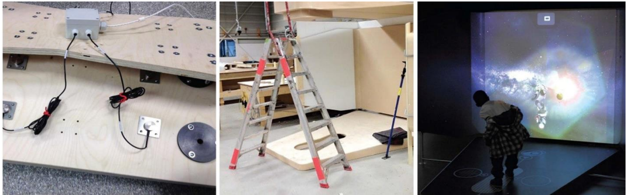
Fig. 8.4.4-3 Left: The sensors mounted on the controller board. The grey box contains the amplification circuitry unit that connects to a pc through a USB. Middle: The exhibit during fabrication; the first time the embodiment design becomes reality, after assembly, it is ready for disassembly and painting. Right: The first participant of the evaluation session, after the construction phase.
