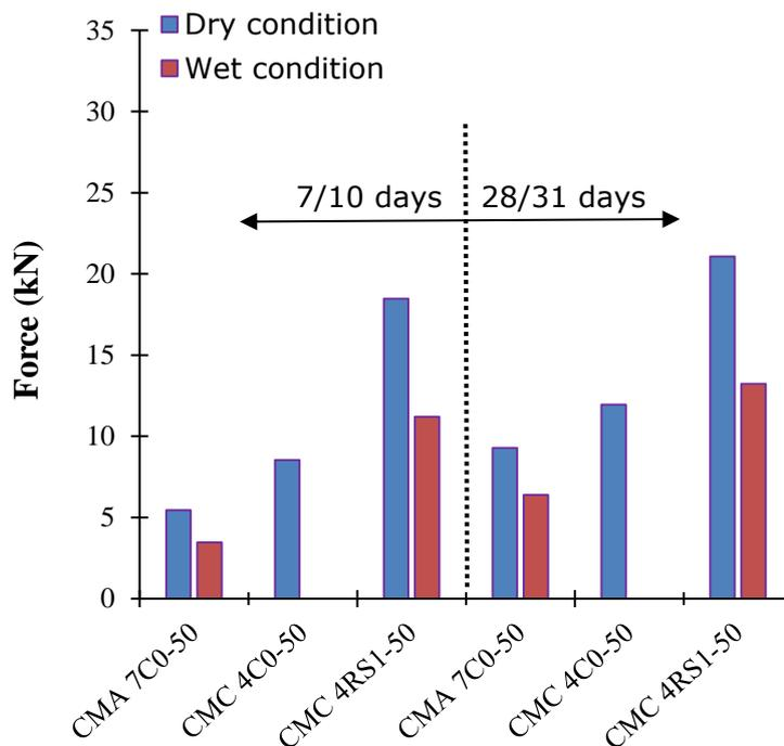
**Figure 5.1** Marshall force resisted measured, at dry and wet conditions, after 7/10 and 28/31 days curing time for the CMA and CMC, with and without cement.
