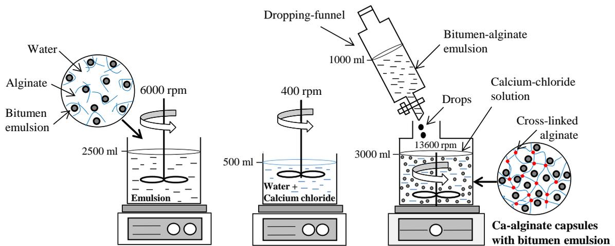
**Figure 3.2** Schematic diagram of the preparation of Ca-alginate capsules containing bitumen emulsion. The procedure is also applicable to the manufacturing of the Ca-alginate particles without bitumen emulsion.
