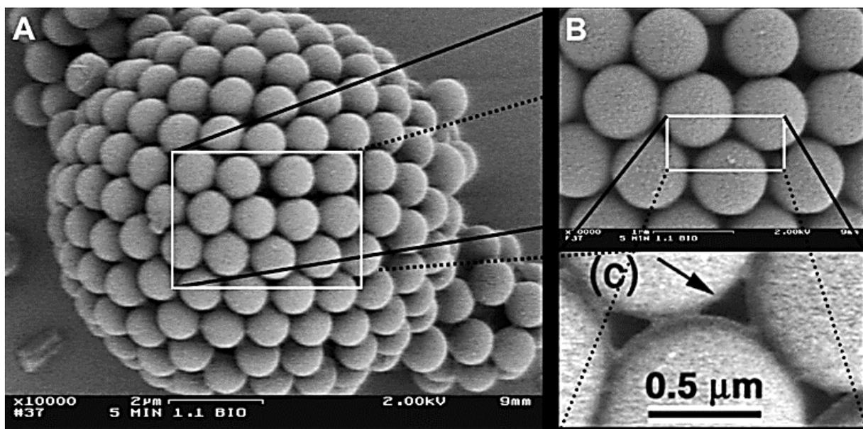
**Figure 2.23** Scanning Electron Microscopy (SEM) images of a typical colloidosome showing (a) the assembly of colloidal particles on the interface of an emulsion droplet and (b) and (c) the pores (open space between particles) that control permeability (Dinsmore et al., 2002).
