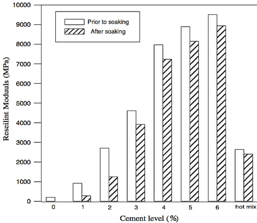
**Figure 2.14** Influence of CMA with different amounts of cement on resistance to water damage (Oruc et al., 2007).
