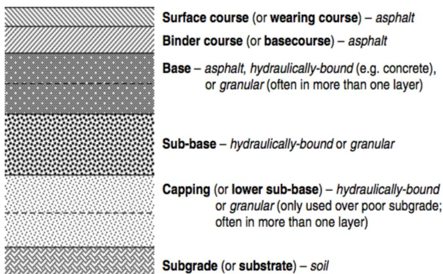
**Figure 2.1** Layers in a typical flexible pavement (Thom, 2008).
