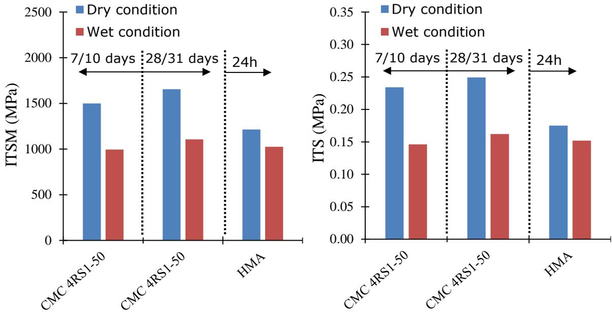
**Figure 6.2** (a) stiffness modulus and (b) indirect tensile strength measured, at dry and wet conditions, after 7/10 and 28/31 days curing time for the CMC 4RS1-50, compared to the HMA specimens, after 24 hours.
