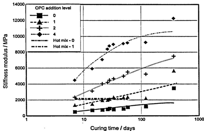
**Figure 2.9** Effect of Ordinary Portland cement (OPC) on stiffness modulus over curing time (Needham, 1996).
