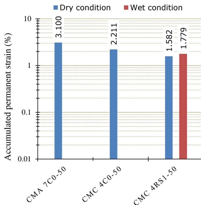
**Figure 5.3** Permanent deformation resisted, at dry and wet conditions, after 28 days curing time for the CMA and CMC, with and without cement, compared to the HMA specimens, after 24 hours.
