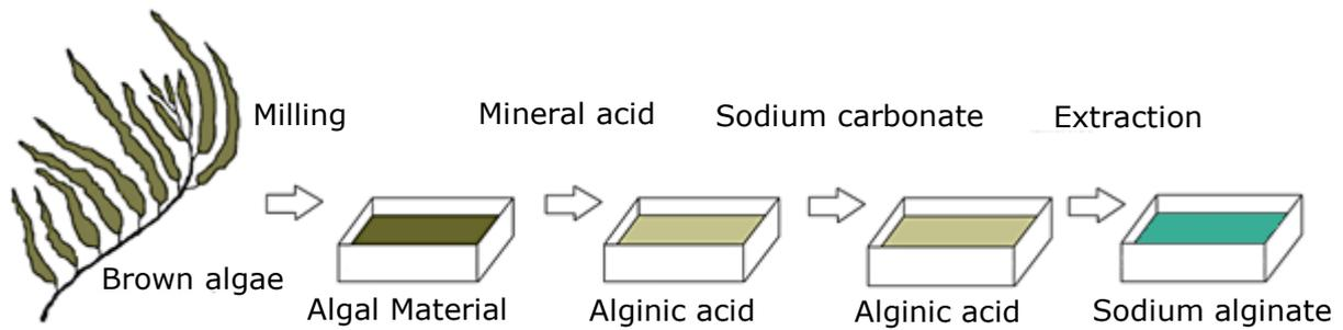
**Figure 2.30** The procedure of sodium alginate extraction from brown algae (Sachan et al., 2009).
