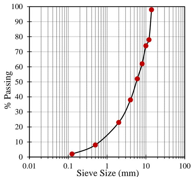
**Figure 3.1** Aggregate size distribution used in the mixture studied.
