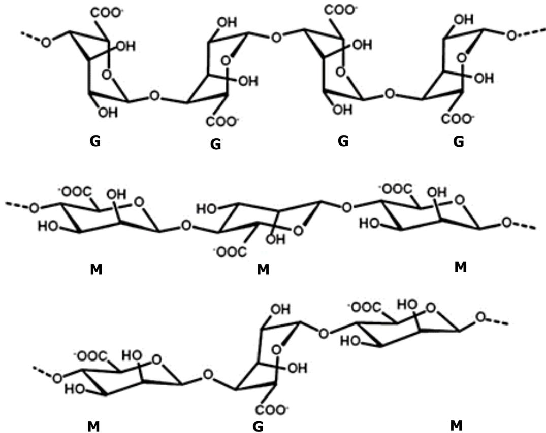
**Figure 2.33** Chemical structures of G, M and alternating blocks in alginate (Lee and Mooney, 2012).
