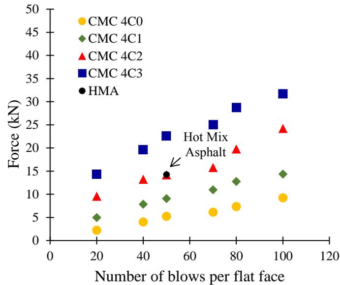
**Figure 3.6** Variations in the Marshall force resisted by CMC test specimens, after 24h curing at 20°C due to the effect of Marshall compaction configurations and Portland cement additions.
