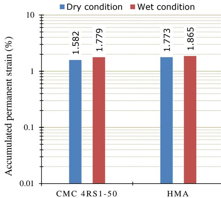
**Figure 6.3** Permanent deformation, at dry and wet conditions, after 28/31 days curing time for the CMC 4RS1-50, compared to the HMA specimens, after 24 hours.
