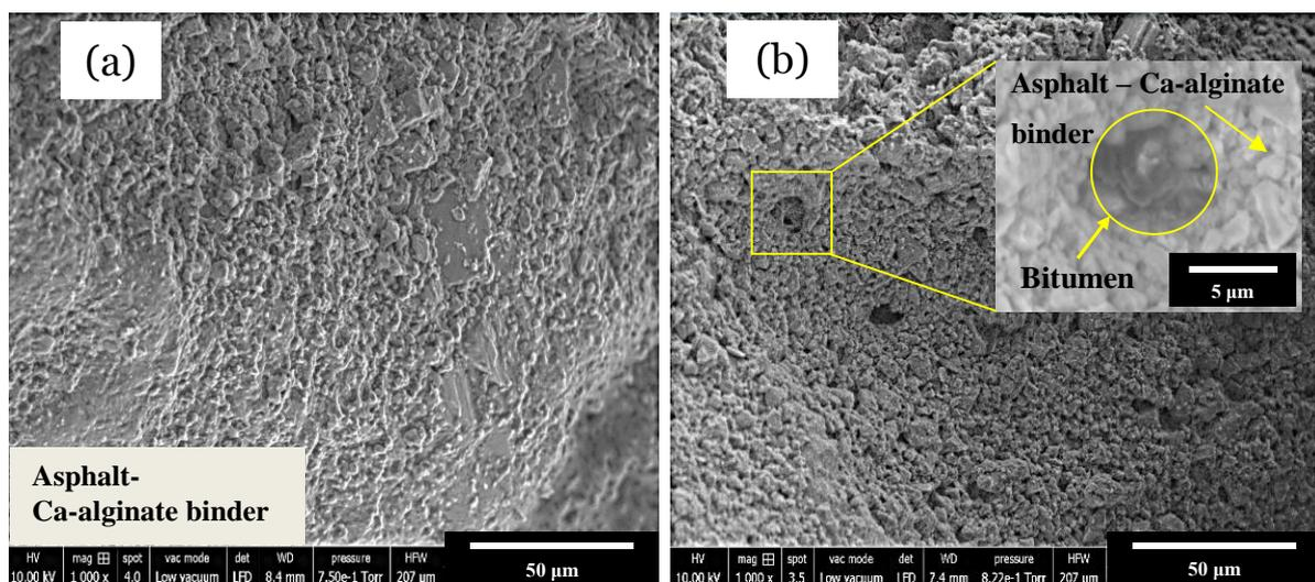
**Figure 3.10** ESEM images of the binder's detail for mixes: (a) CMP 4C0-50 and, (b) CMC 4C1-50.
