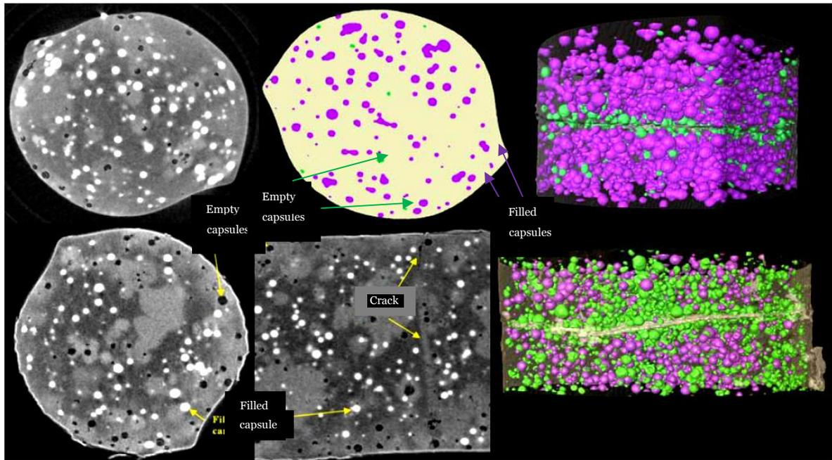
**Figure 2.28** CT scan image of self-healing polymer through material (capsules) (Mayo et al., 2012).
