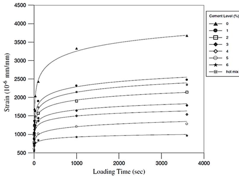
**Figure 2.10** Effect of different cement content on CMA permanent deformation resistance (Oruc et al., 2007).
