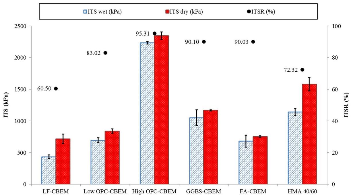
**Figure 2.15** Moisture damage at different additives content on CMA (Nassar et al., 2016).
