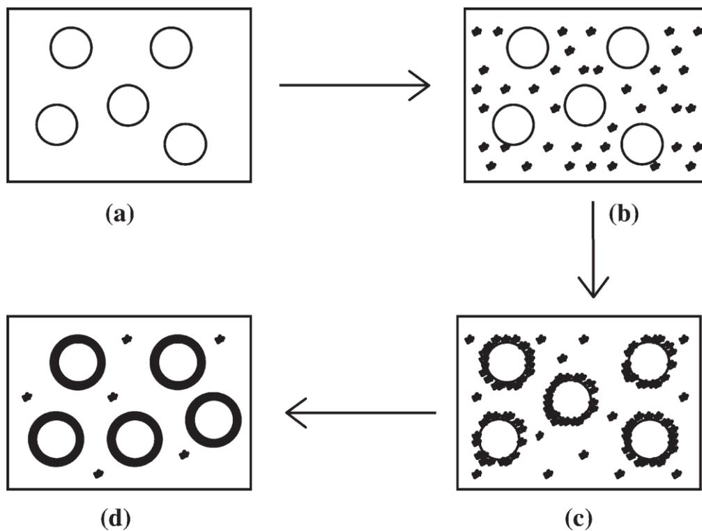
**Figure 2.21** Schematic representation of the coacervation process: (a) Core material dispersion in shell polymer solution; (b) Coacervate separation from solution; (c) Coating of core material (d) Coalescence of coacervate to form continuous shell (Redrawn from Jyothi et al., 2010).
