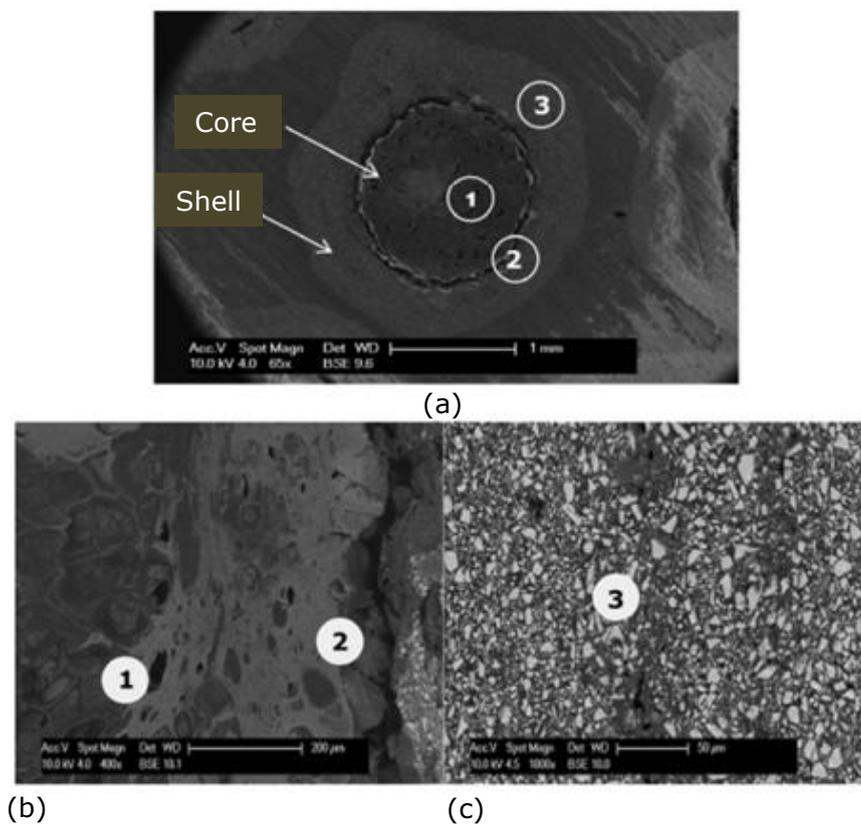
**Figure 2.29** SEM images of capsule; (a) overview of the capsule; (b) zoom-in of the core and the core-shell interface; (c) zoom-in of the shell (Al-Mansoori et al., 2016).
