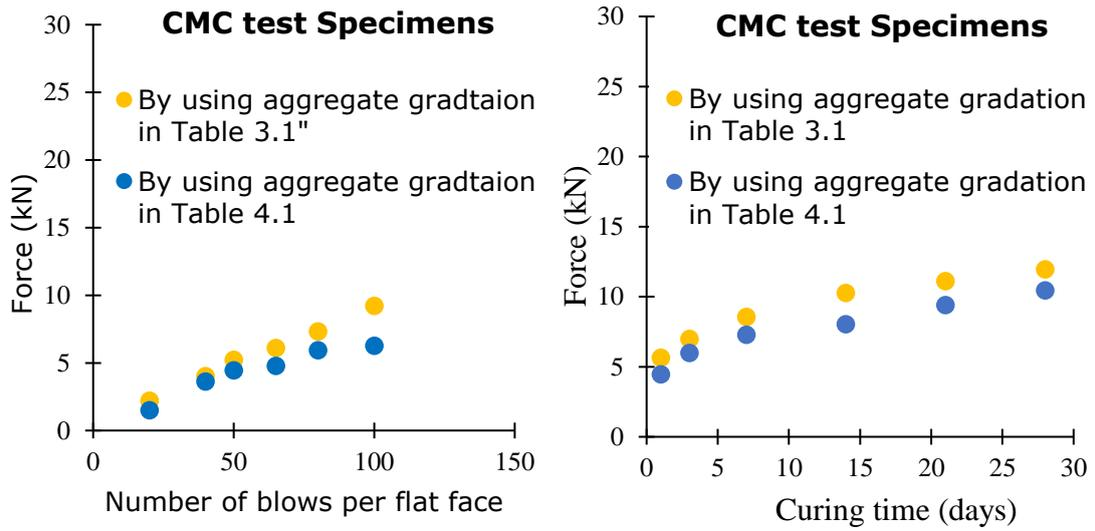
**Figure 2** Marshall force registered for CMC test specimens, , at 20°C by using aggregate gradation in Table 3.1 and Table 4.1 (a) at different number of blows per flat face, after 24 curing, and (b) at different curing times.
