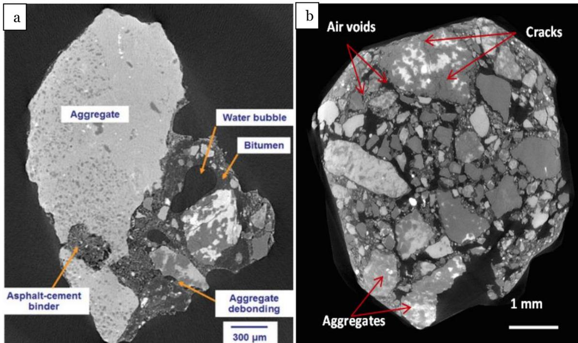
**Figure 2.13** (a) Micro CT image of a cement and asphalt composite (García et al., 2013) and (b) Micro tomography detail of CMA (Fang et al., 2016).
