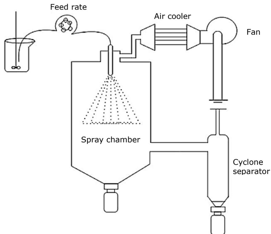
**Figure 2.20** Scheme of spray cooling equipment (Okuro et al., 2013).
