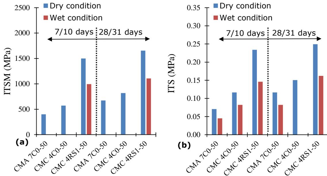
**Figure 5.2** (a) stiffness modulus and (b) indirect tensile strength measured, at dry and wet conditions, after 7/10 and 28/31 days curing time for the CMA and CMC, with and without cement.
