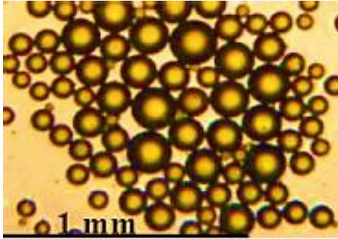
**Figure 2.26** Chitosan Microcapsules Microphotograph. The microcapsules were made at 0.5wt% natural coconut oil, 0.5wt% NaOH, and 0.5wt% Chitosan at a stirring rate of 800 rpm (Hsieh et al., 2006).
