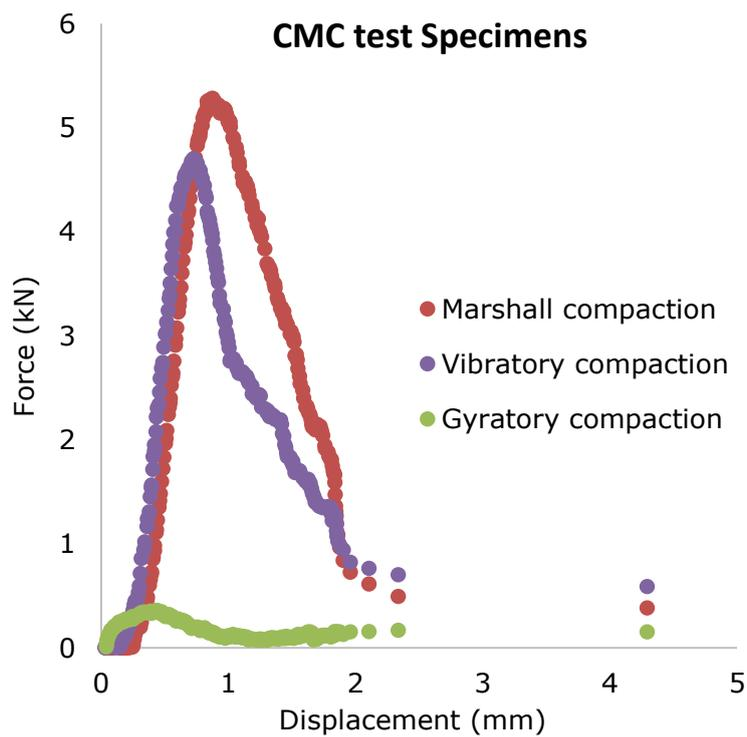
**Figure 1** Marshall force registered for CMC test specimens, at 20°C by using aggregate gradation in Table 3.1, after 24 curing.
