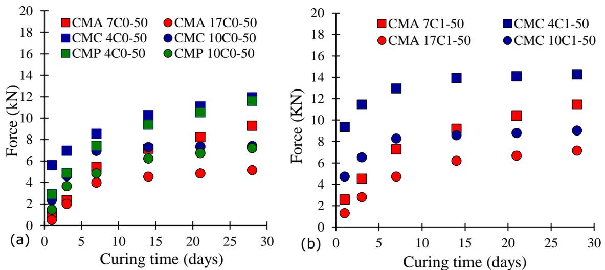
**Figure 3.9** Marshall force registered at different curing times for (a) CMA, CMC and CMP without cement, and (b) CMA and CMC with 1% Portland cement.
