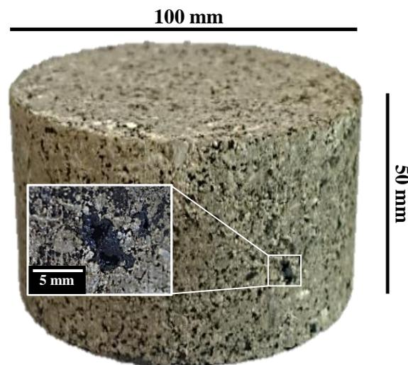
**Figure 3.4** Test specimen of cold mix pavement made with Ca-alginate with bitumen emulsion.
