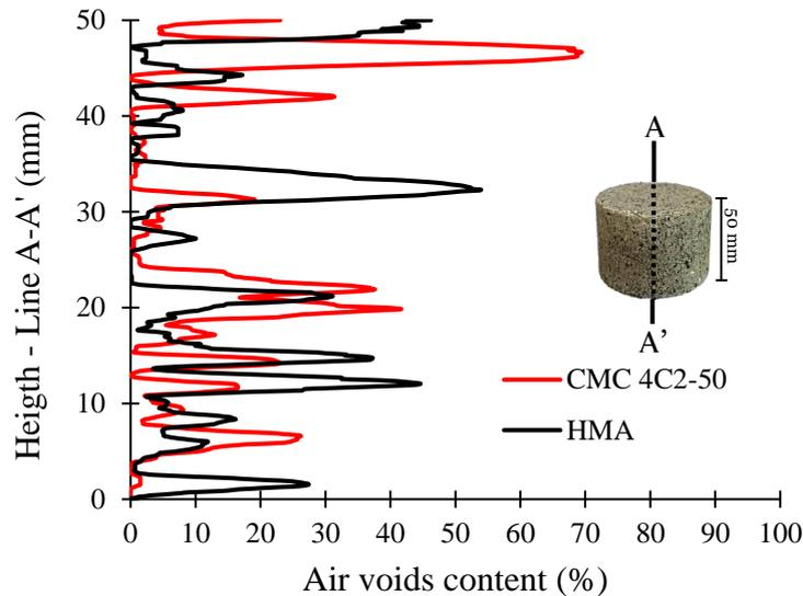
**Figure 3.7** Air voids distribution along the vertical axis of CMC 4C2-50 and HMA test samples.
