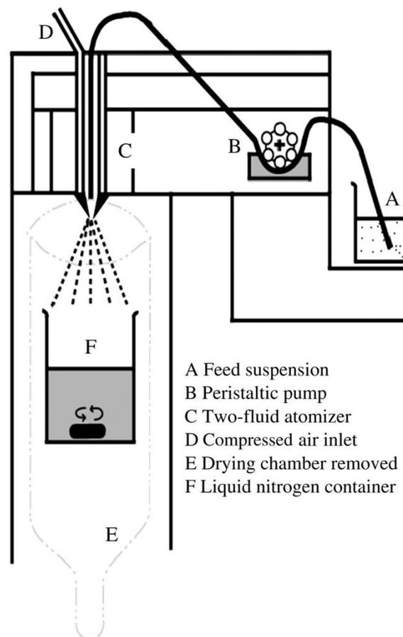
**Figure 2.22** Schematic diagram of spray freeze drying method (Kho and Hadinoto, 2011).
