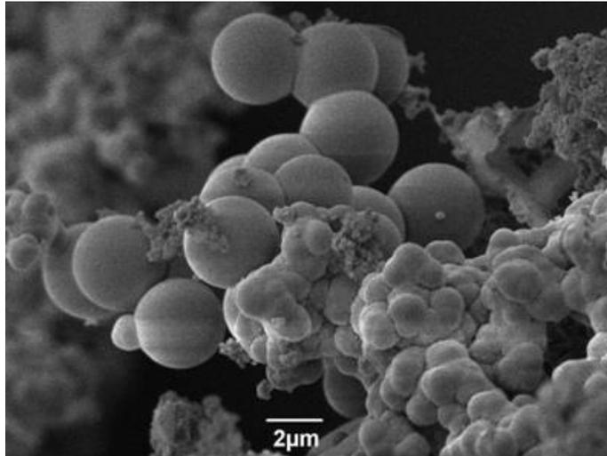
**Figure 2.18** Matrix microcapsules containing silica (AZoMaterials, 2013).
