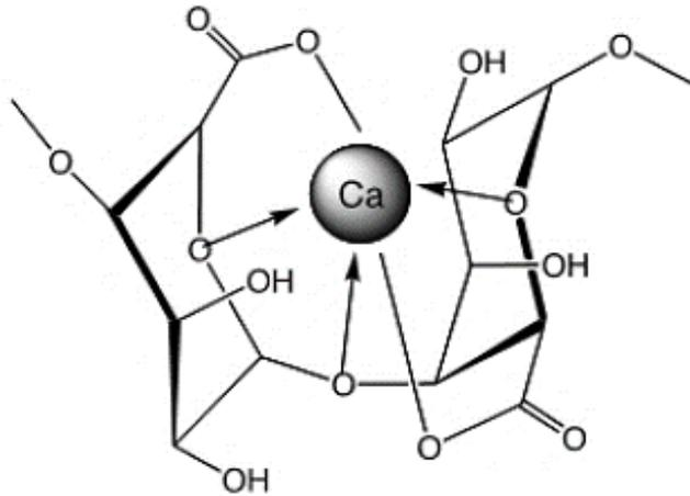
**Figure 2.34** Egg-Box structure of calcium alginate structure (Inoue et al., 2018).
