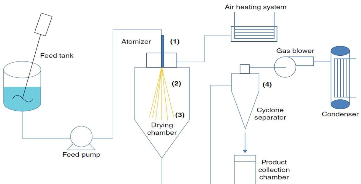
**Figure 2.19** Spay drying process: (1) Atomization (2) Spray – hot air contact (3) Evaporation of moisture (4) Product separation (Anandharamakrishnan, 2015).
