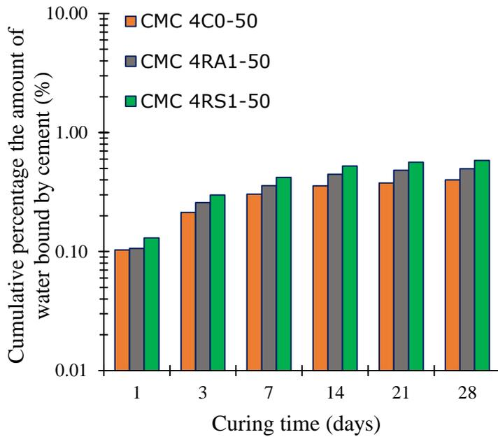
**Figure 4.6** Amount of water bound measured at different curing time for CMC 4C1-50, CMC 4RA1-50 and CMC 4RS1-50.
