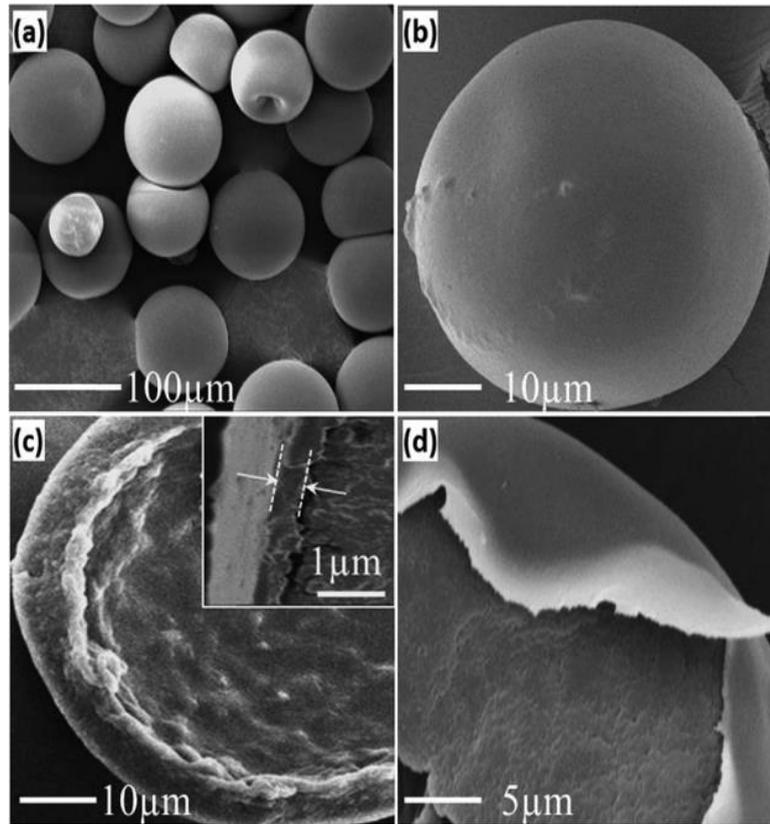
**Figure 2.25** SEM images of double-layered polyurea microcapsules containing hexamethylene diisocyanate (HDI) (Sun et al., 2012).
