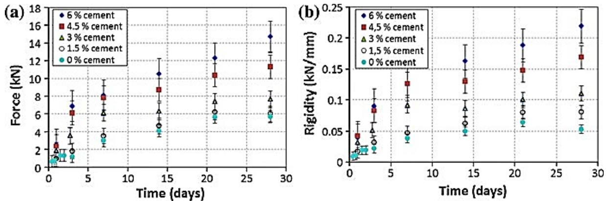
**Figure 2.11** a) Marshall strength (kN) with time and b) Rigidity (kN/mm) with time, for CMA with different amounts of Ordinary Portland cement (OPC) cured at 90 % environmental humidity (García et al., 2013).
