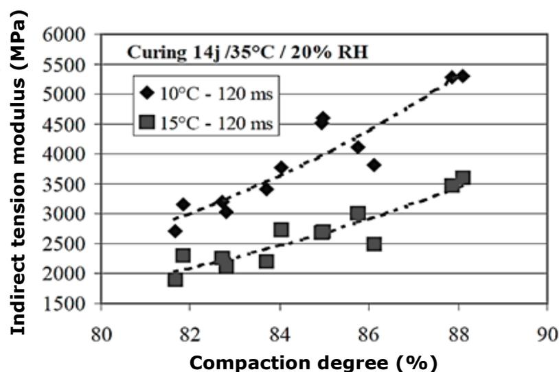
**Figure 2.8** Effect of compaction degree on stiffness modulus of CMA (Serfass et al., 2004).
