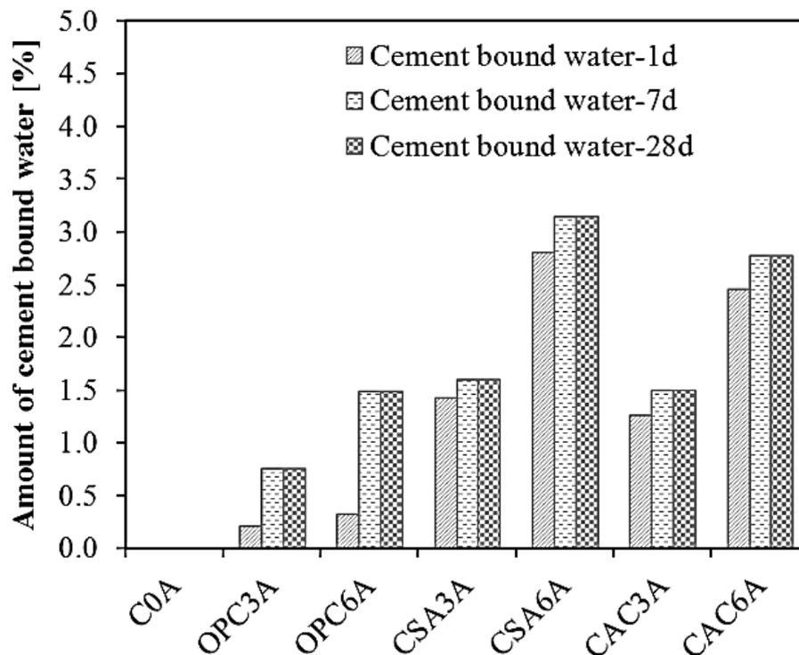
**Figure 2.12** Amount of water bound for the CMA specimens with 0%, 3% and 6% of Ordinary Portland cement (OPC), calcium aluminate cements (CAC) and calcium sulfoaluminate cements (CSA), after 1, 7 and 28 days curing (Fang et al., 2016).
