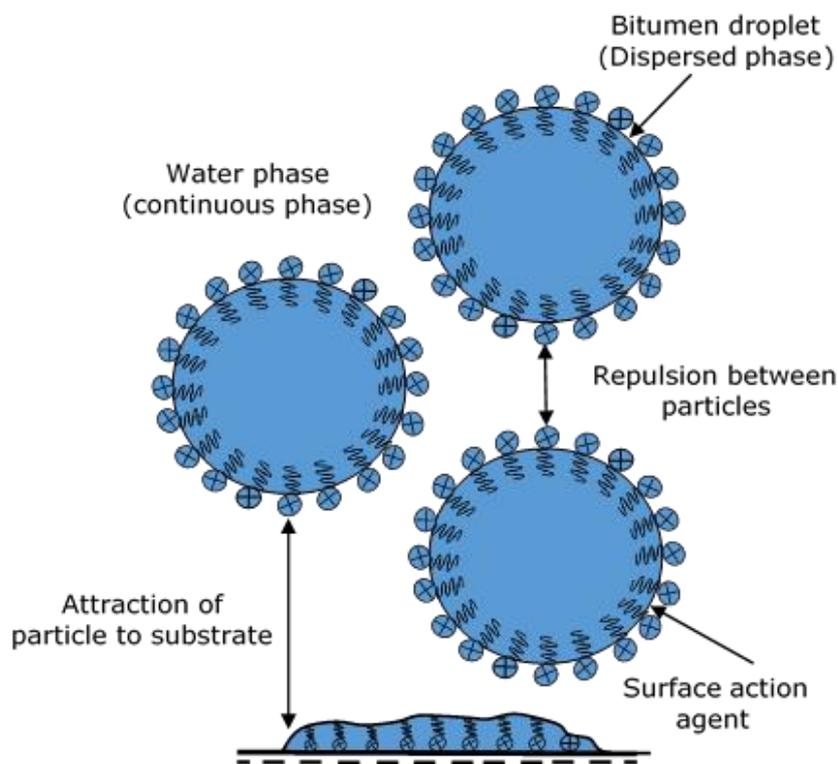
**Figure 2.5** Schematic diagram of bitumen during dispersion in an emulsifier (Read and Whiteoak, 2003).
