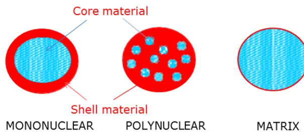
**Figure 2.16** Types of microcapsules (Bevilacqua et al., 2010).
