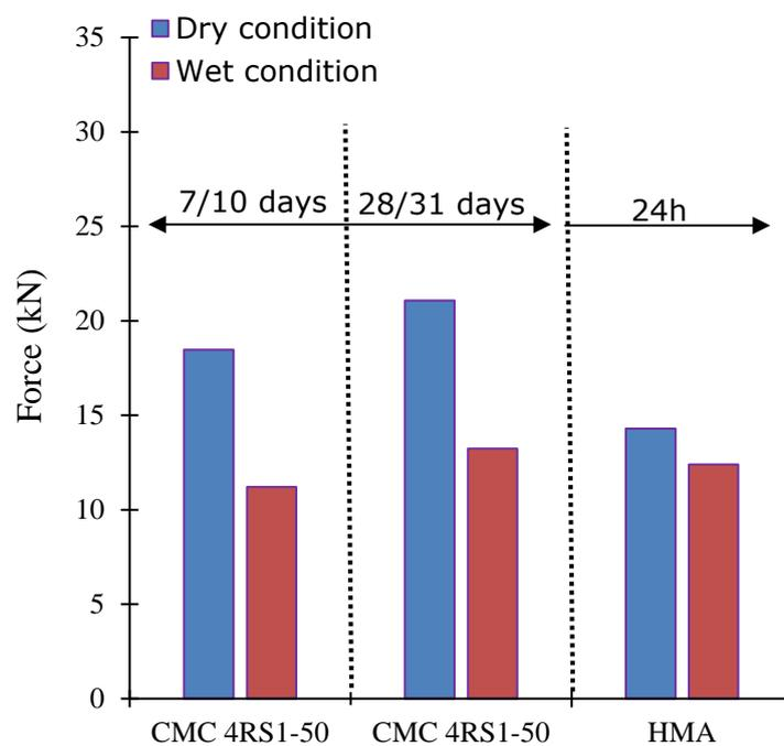
**Figure 6.1** Marshall force resisted measured, at dry and wet conditions, after 7/10 and 28/31 days curing time for the CMC 4RS1-50, compared to the HMA specimens, after 24 hours.
