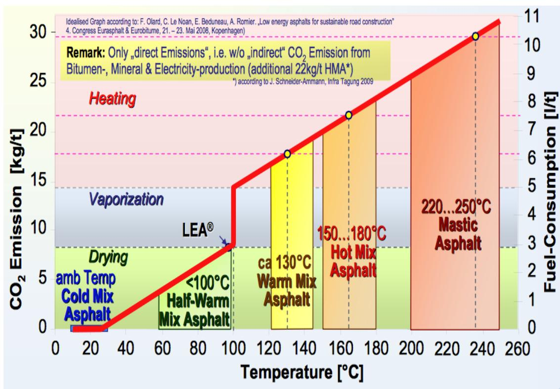
**Figure 2.3** The CO<sub>2</sub> emissions and energy consumption (Partl, 2010).
