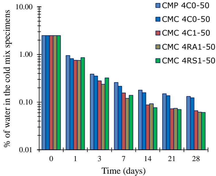
**Figure 4.5** Water content measured at different curing times for CMC specimens with and without 1% of cement.
