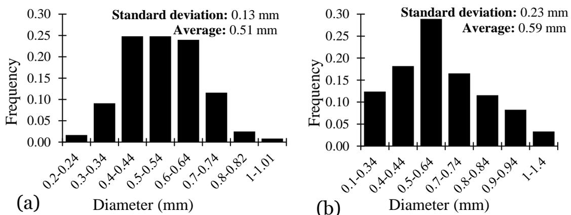
**Figure 3.5** Sizes distribution of: (a) Ca-alginate capsules, see Figure 3(a), and (b) Ca-alginate particles, see Figure 3(b).
