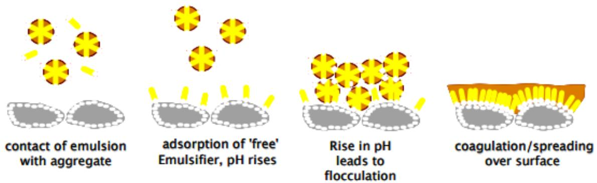
**Figure 2.7** Stages in the breaking of a cationic emulsion (James, 2006).
