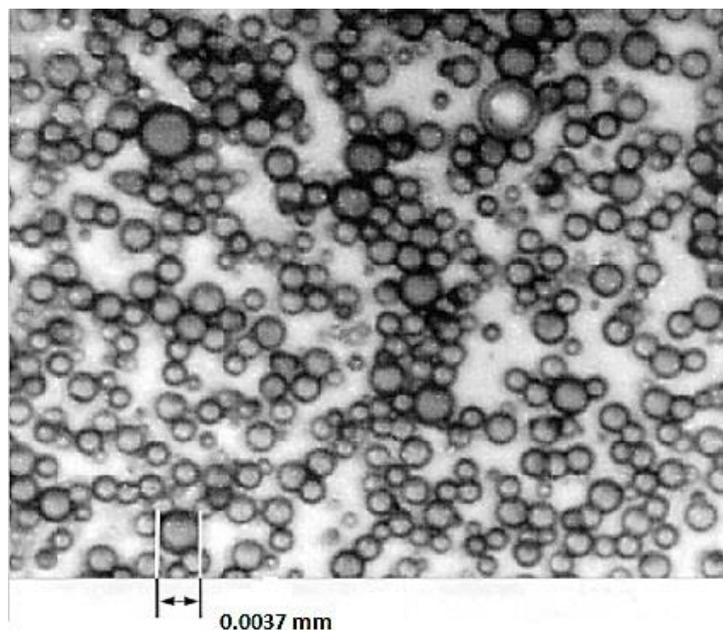
**Figure 2.6** Bitumen droplets in an emulsion and their relative size (Chemarc, 2017).
