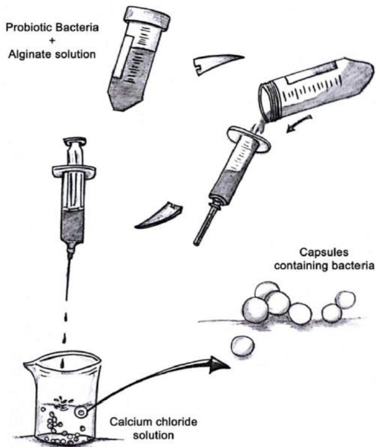
**Figure 2.24** Schematic diagram of the extrusion encapsulation method (Serna-Cock and Vallejo-Castillo, 2013).
