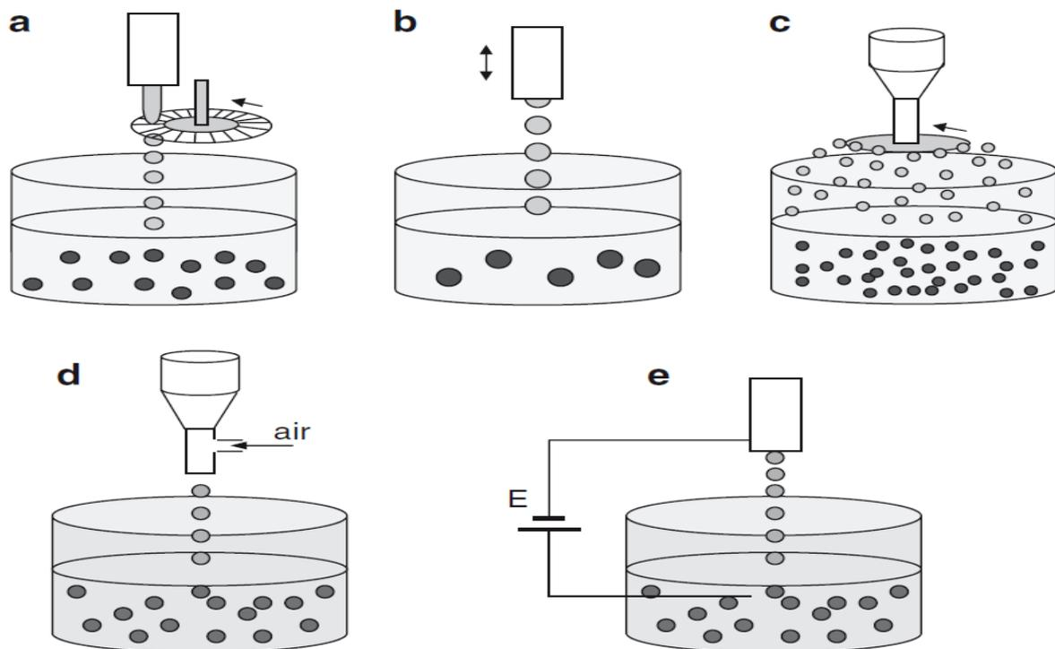
**Figure 2.32** Set-ups of five different ways of making microspheres: (a) Jet Cutter , (b) pipette or vibrating nozzle (c), atomizing disk (d), coaxial air-flow (e) electrostatic potential (Zuidam and Nedoviæ, 2010).
