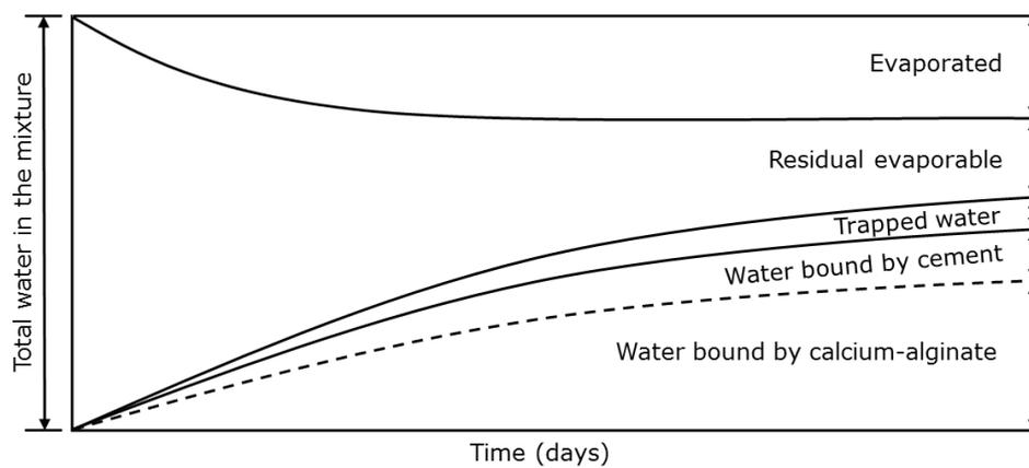
**Figure 4.2** Schematic diagram for the distribution of water in the total CMC with cement addition.
