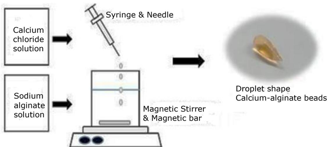
**Figure 2.31** Encapsulation process of calcium-alginate beads (Sewiwat et al., 2016)
