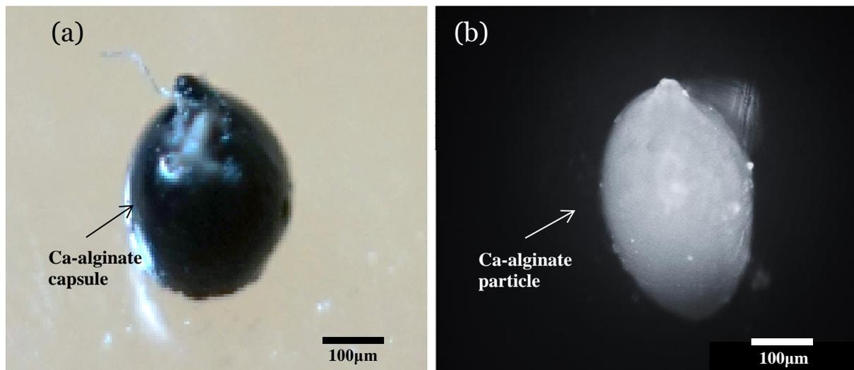
**Figure 3.3** (a) Optical image of an individual Ca-alginate capsule containing bitumen emulsion. (b) Fluorescence image of an individual Ca-alginate particle without bitumen emulsion.
