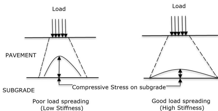
**Figure 2.2** Pavement stiffness and load spreading through asphalt layers (Brown, 1988).
