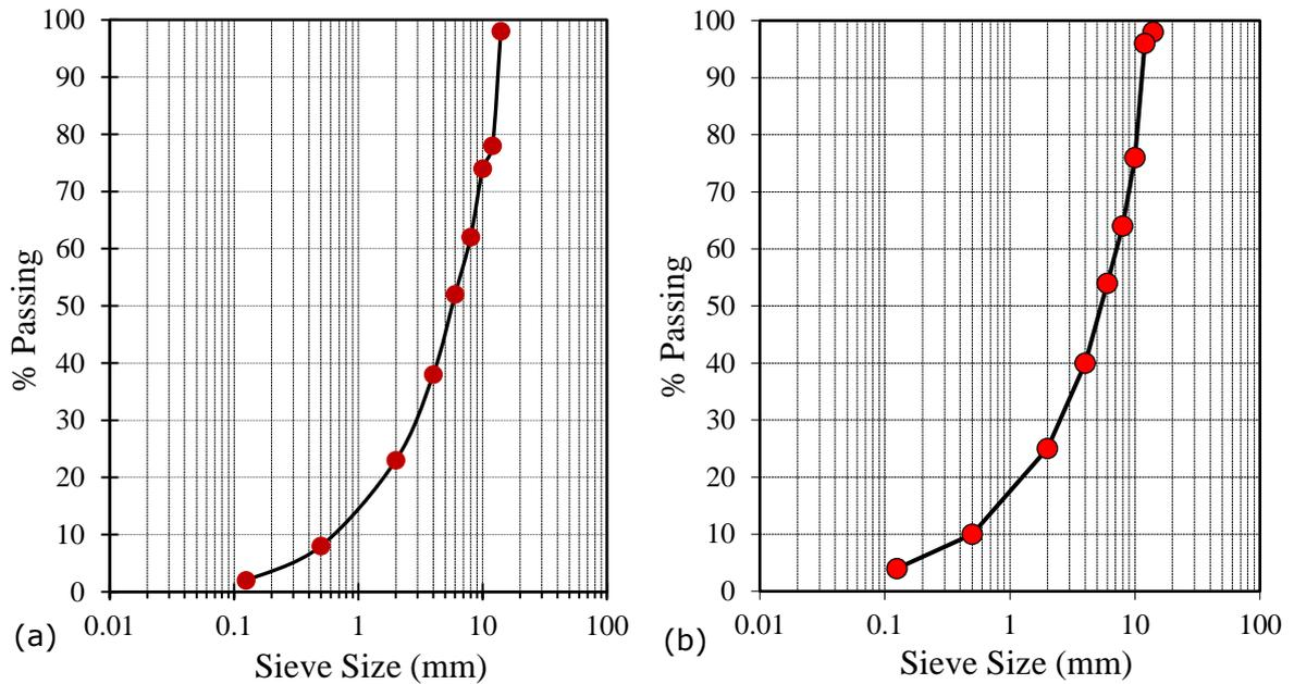
**Figure 4.1** Aggregate size distribution used in (a) Chapter 3, and (b) Chapter 4.
