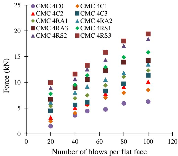
**Figure 4.3** Variations in the Marshall force resisted by CMC test specimens, after 24h curing at 20°C due to the effect of Marshall compaction configurations and rapid cement addition as well as Portland cement addition.
