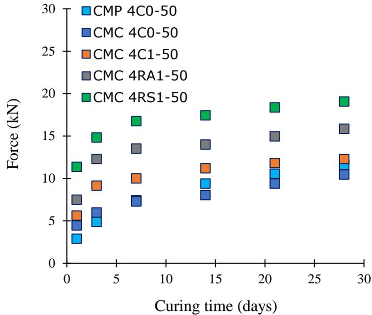
**Figure 4.4** Marshall force resisted measured at different curing times for CMC specimens, with and without 1% of cement.
