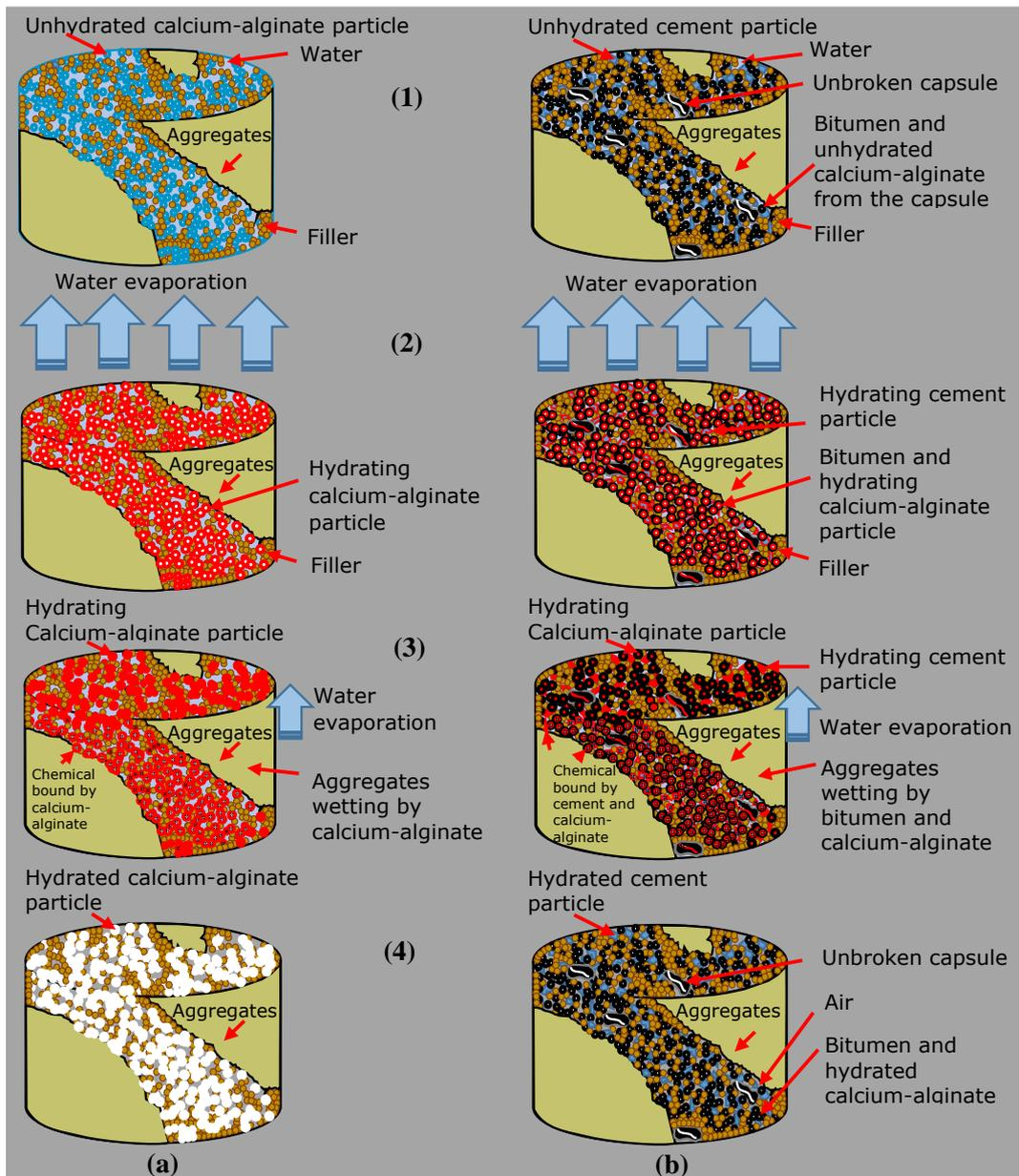
**Figure 4.7** Schematic representation of the hydration process for (a) CMP without cement (b) CMC with cement.
