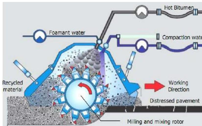
**Figure 2.4** Foamed Asphalt application for cold pavement recycling (Ebels et al., 2005).
