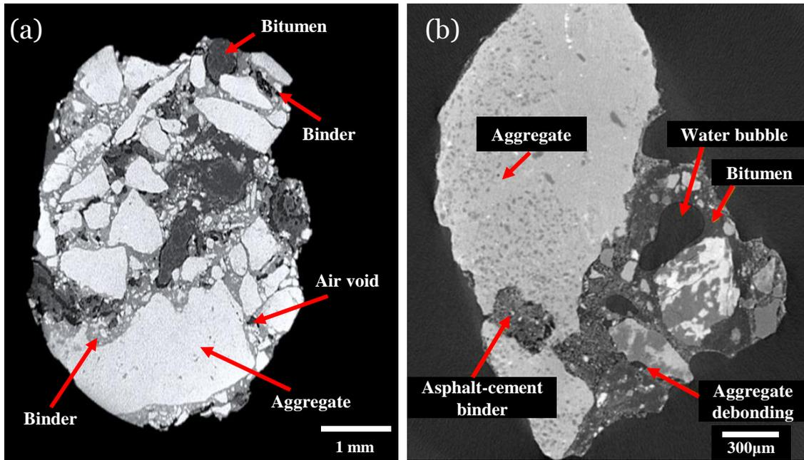
**Figure 3.8** (a) CT-Scan detail of a cold mix pavement material sample CMC 4C2-50, cured for 28 days. (b) CT-Scan detail of a CMA, taken from a test sample, cured for 28 days, with 6% of cement (modified from Garcia et al. 2013).
