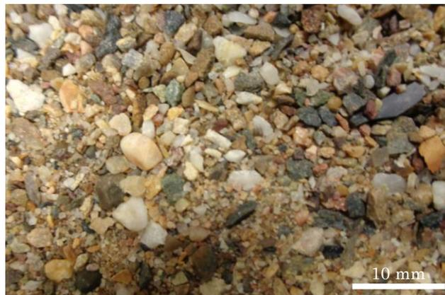
Figure 2.5: Mineral aggregates in the size range for asphalt mortar, which comprises of fine aggregates and filler.
