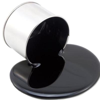
Figure 2.1: Bitumen flowing out of a tin, due to gravity. The high viscosity of bitumen is responsible for spilling of bitumen at ambient temperature taking a long time [42].
