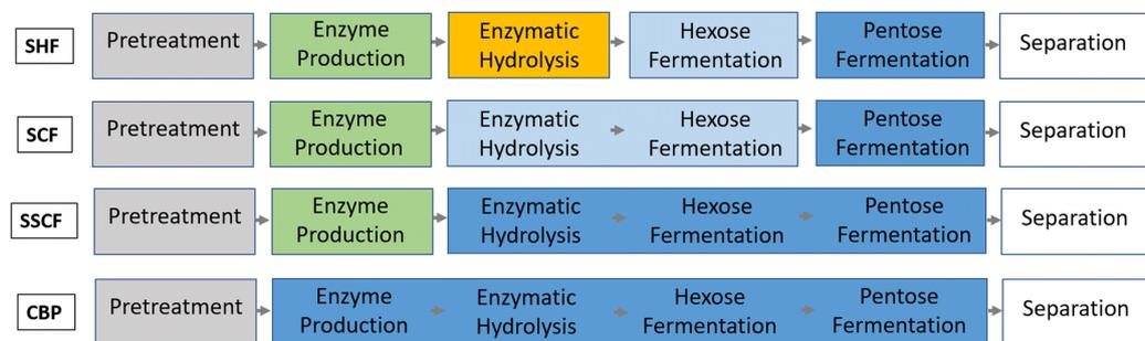
**Figure 1. 6:** Types of bioprocessing for solvent production from lignocellulose.
