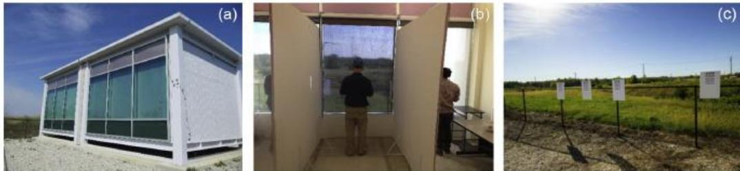
**Figure 2-8.** (a) Exterior view of test offices (left), (b) interior partitioning (middle), and (c) Landolt C boards installed outside (right) [45].
