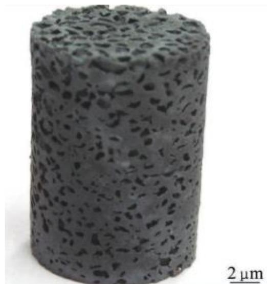
*Figure 2.12. Ti-Co Foam Manufactured by the Space Holder Sintering Process [70]*
