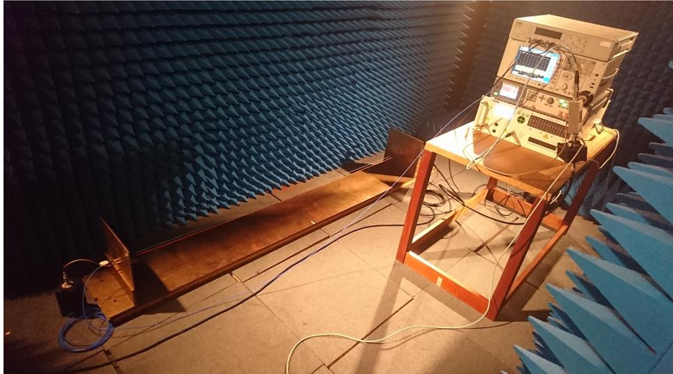
Figure 5.13: Photograph of the interior of the anechoic chamber for crosstalk measurements.
