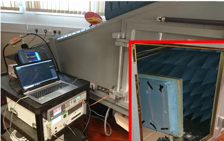
Figure 5.5: Complete experimental setup for GTEM measurements.
