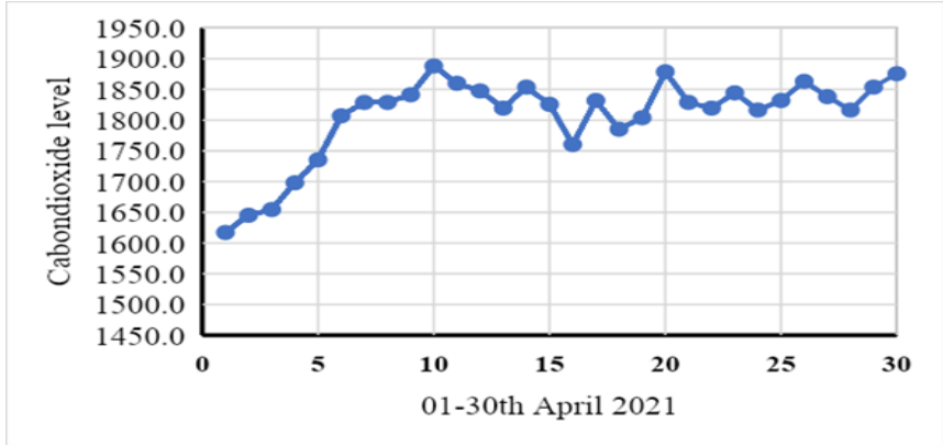
Figure 5-6 Indoor Carbon dioxide (CO 2 ) measurement in the classroom in April.
